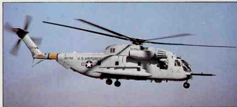
The USAF Aerospace Rescue and Recovery Service uses the HH-53B and HH-53C, with extensive special mission equipment including a flight refuelling probe. This example was photographed with landing gear extended
