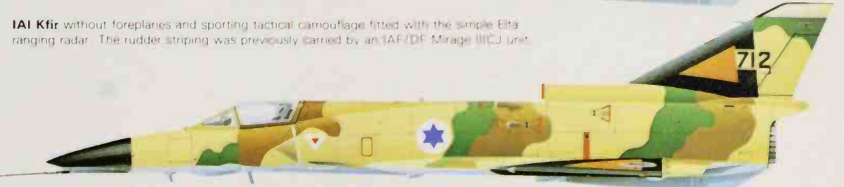
This Kfir is one from the initial production batch, demonstrated in public at Hatzorim airbase in August 1976, together with the first Kfir-C2 with canard foreplanes. Fitted with the definitive radar, it was subsequently brought up to C2 standard.
