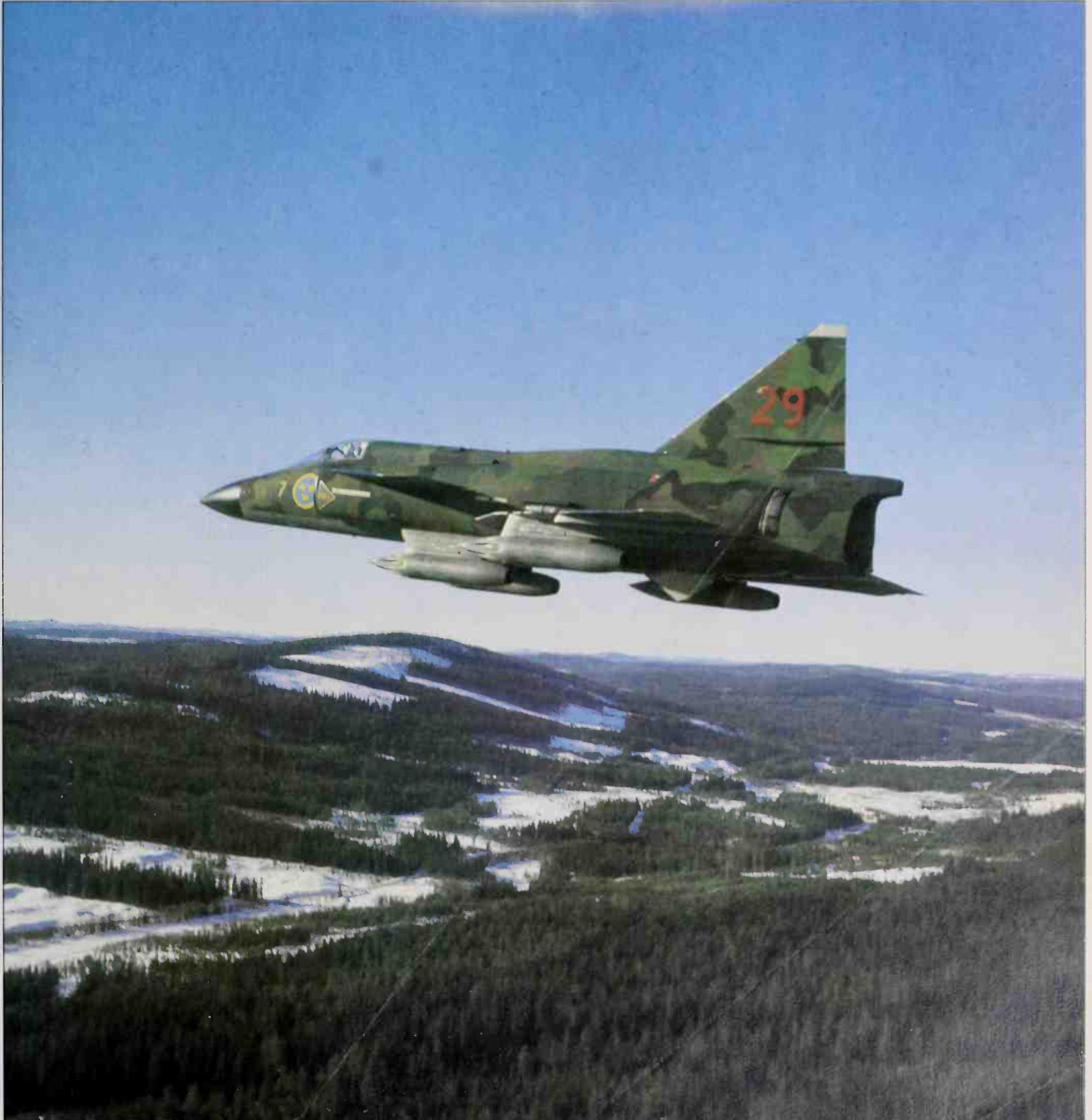
First user of the AJ37A attack Viggen was F7 wing at Sätenas whose three squadrons were all fully equipped with the extremely effective new aircraft by the end of 1975. This example is seen carrying four pods of Bofors spin-stabilized rockets (each housing six 135mm projectiles).
