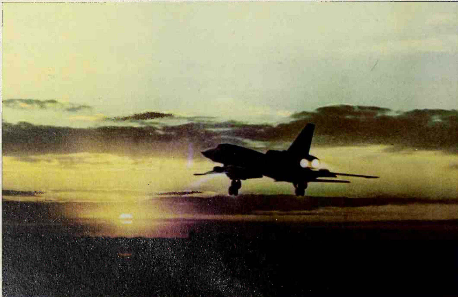
A frame from a Soviet propaganda film showing dusk takeoff of a Tu-22 supersonic reconnaissance platform of the Soviet naval air force (AV-MF). The sub-type cannot be identified but it is probably a so-called 'Blinder-C' with extensive cameras and other sensors and comprehensive ECM systems. Gross weight is 185,000 lb (83,900 kg).
