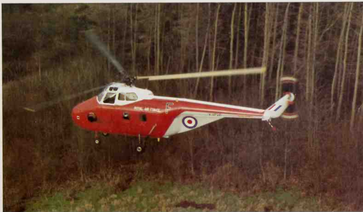
The RAF's Whirlwind HAR.10, of which this (XJ726) is a colourful example, is by far the best of all the many versions of the S-55 of 1949. Powered by a Gnome turboshaft, they have many airframe and systems improvements. This one is a trainer at Shawbury.
