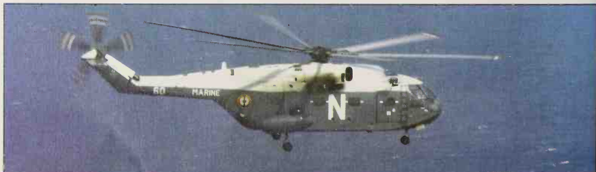
France's Aéronautique Navale uses the big Super Frelon in both the ASW and Commando assault-transport roles.
