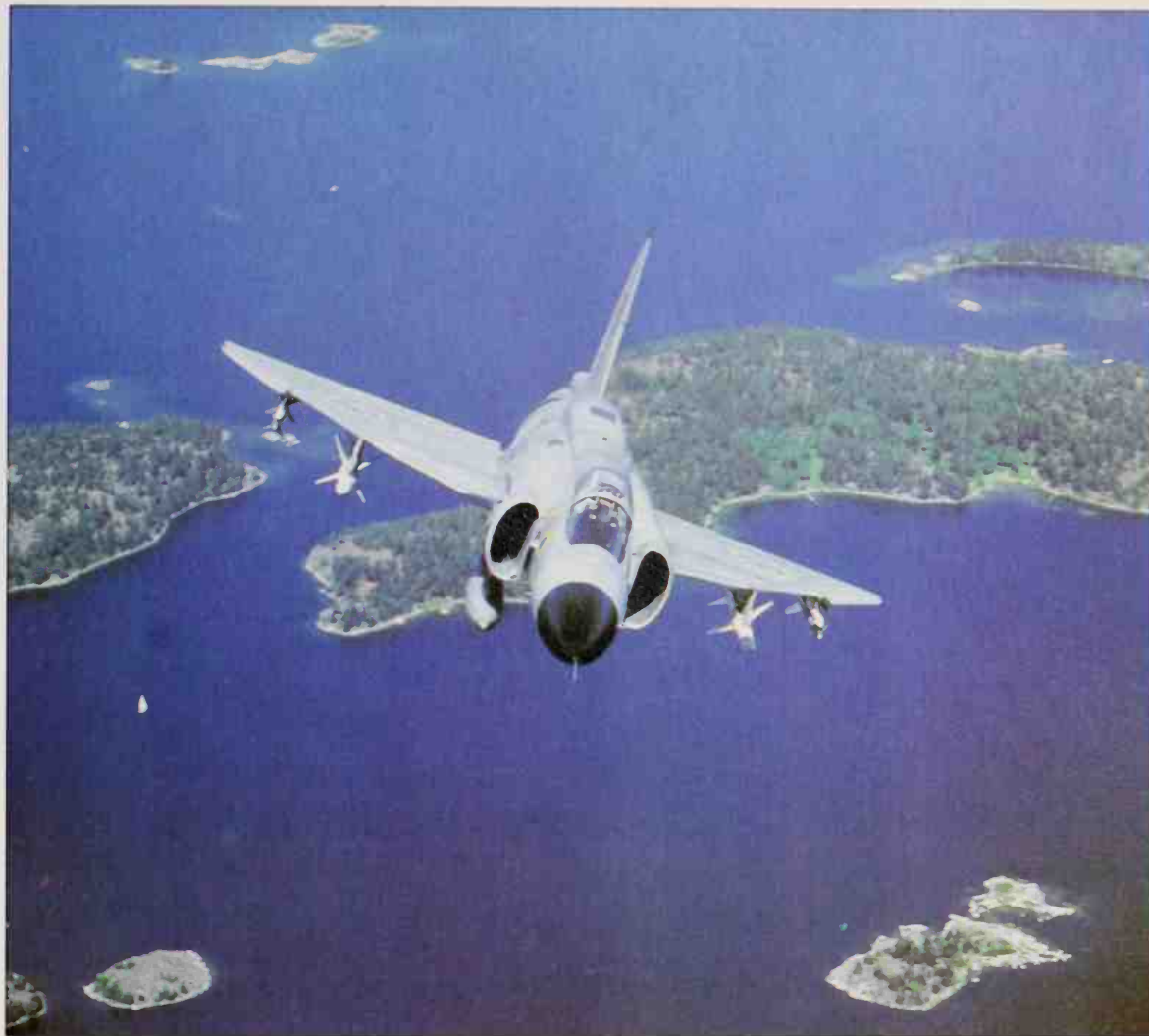
Now in the early stages of operational service with Sweden's Flygvapen the Saab JA37 Viggen interceptor has outstanding all-round performance, advanced Ericsson pulse-doppler radar and Sky Flash medium-range missiles. Swedish AIM-9s are outboard
