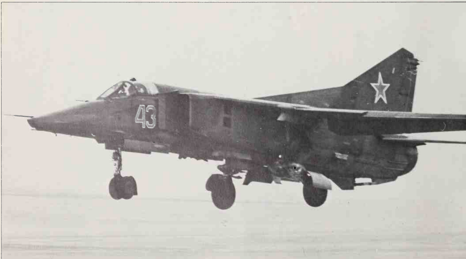
Landing after a sortie, this Soviet FA MiG-27 'Flogger-D' has its flaps fully down on the wings in minimum-sweep position, and the ventral fin folded to the right. Unlike most NATO air forces the FA regiments often operate for prolonged periods from rough unpaved temporary bases, thus giving an outstanding dispersion capability.
