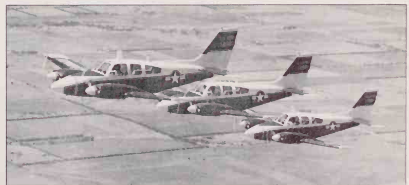
Standard twin-engine fixed-wing trainer of the US Army, the T-42A Cochise is a close relative of the civil Beech Baron, bought off the shelf but fitted with Army communications and additional navids and avionics. A total of 60 are in use.
