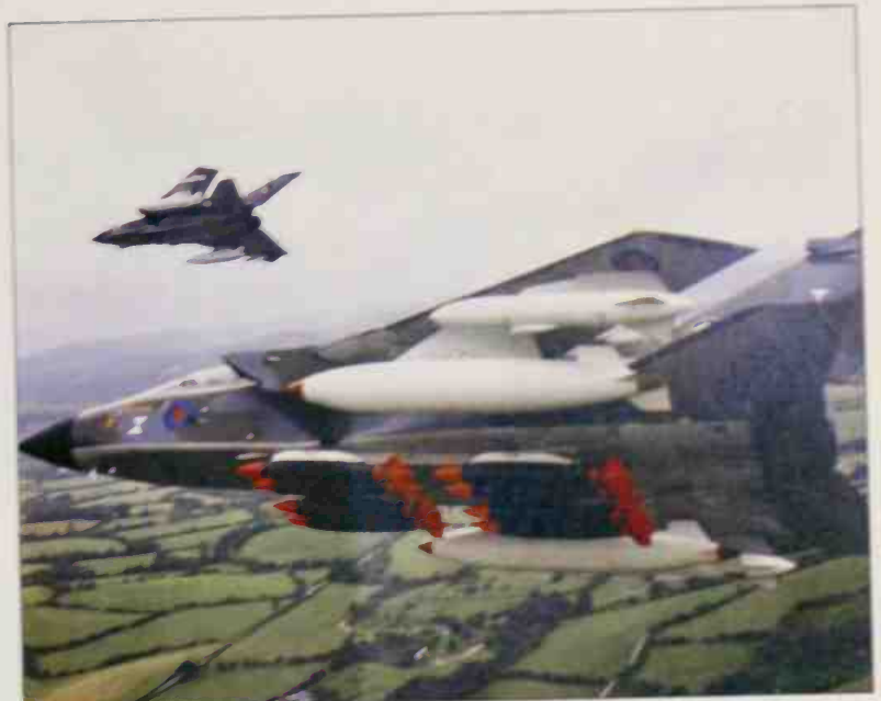
The Panavia Tornado IDS in the foreground is carrying eight bombs of 1,000 lb (454 kg), two large tanks and the new Ajax ECM pods outboard
