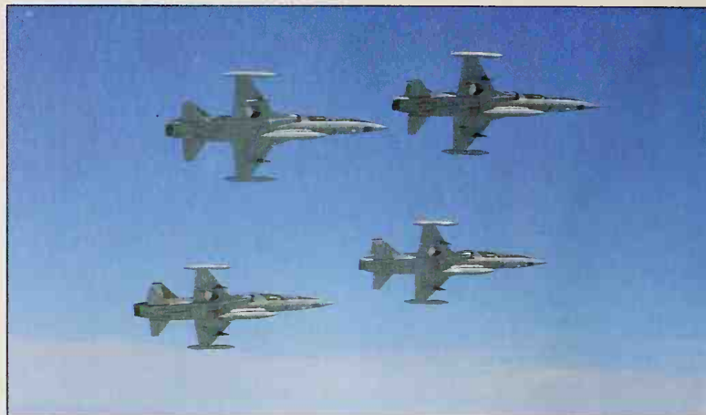
Standard tac-recon types of the KL (Royal Netherlands AF) are the RF-104G and Dutch/Canadian NF-5 Freedom Fighter. These are NF-5As with recon pods.
