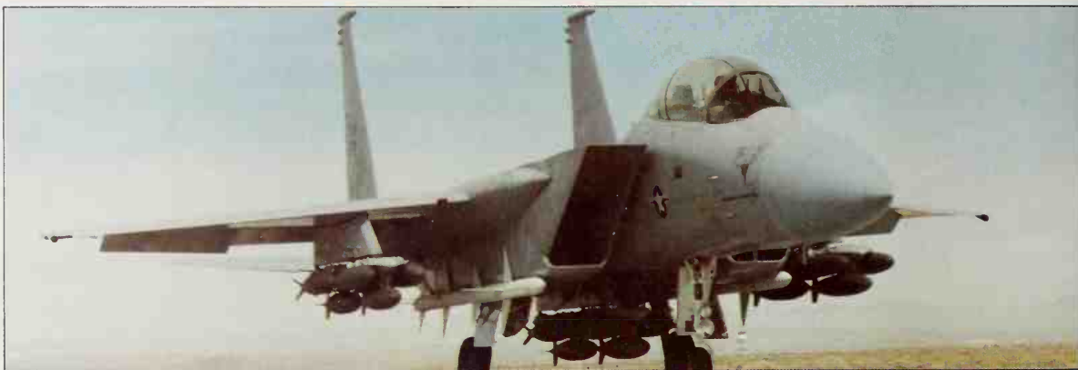
In all configurations, as here with 18 conventional bombs, the F-15 Eagle retains its primary load of four Sparrows.
