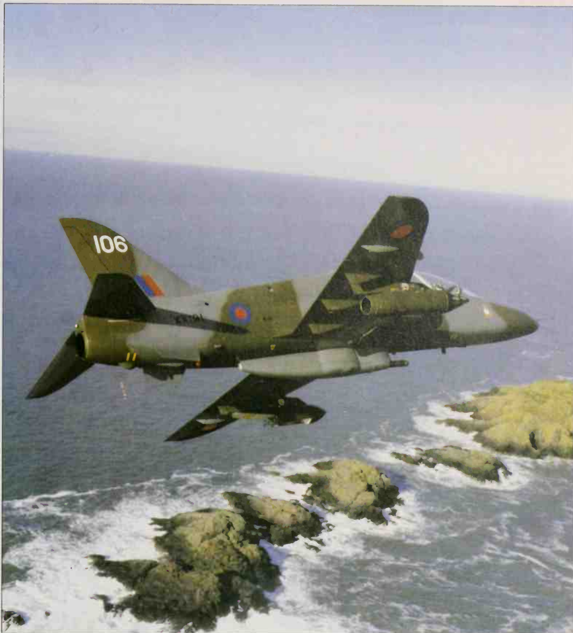
British Aerospace Hawk T.1 of the RAF Tactical Weapons Unit at Brawdy is seen on a rocketing mission off the Welsh coast. Capable of carrying 6,500 lb (2948 kg) of weapons, the Hawk is a powerful tactical platform. By January 1980 the RAF had 160.
