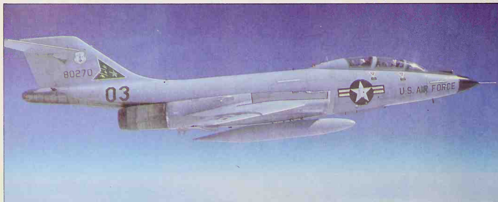
This well-preserved Voodoo is an F-101B still serving as an all-weather interceptor, the unit being the 123rd FIS, Oregon Air National Guard. It was photographed in late July 1977 during Exercise 'Overview', testing the efficiency of the USAF's new E-3A Sentry.
