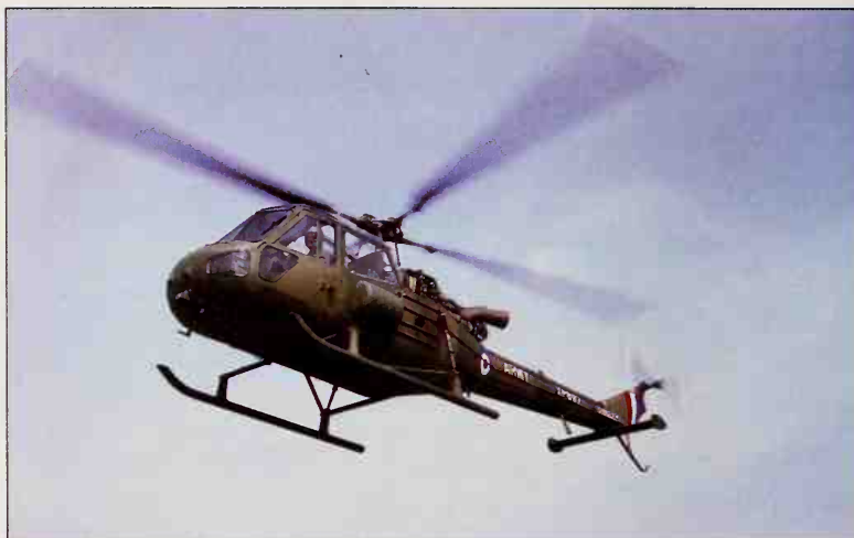
The Westland Scout AH.1, of which 120 were deployed, has been the British army's chief helicopter but is now being replaced by 100 Lynx. This Scout, XP897, has a new paint job and fin insignia, but lacks the pylons and roof sight for missiles.
