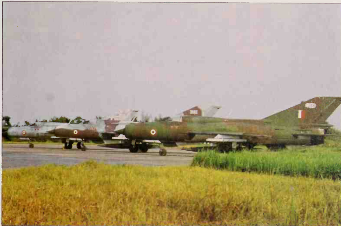
Though showing a complete absence of planning in their colour schemes, these HAL Type // (basically the MiG-21FL built under licence) fighter/bombers are tailored to the Indian AF's needs. Since 1973 HAL has built the later Type 96 and MiG 21bis.
