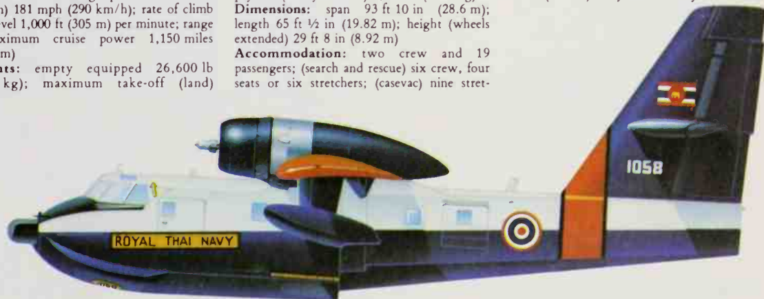
One of two Canadair CL-215 amphibians delivered to the Royal Thai Navy in 1978 and operated from Bangkok on search and rescue duties.
