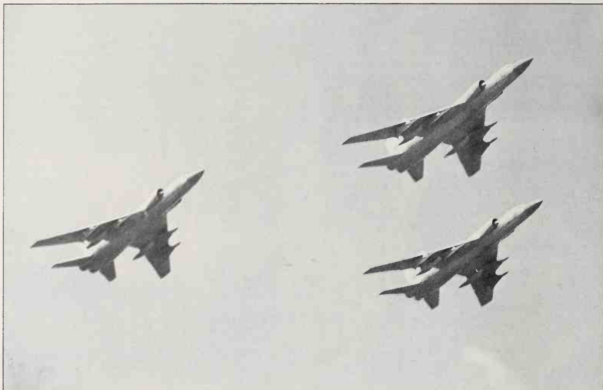
Three of the world's biggest fighters, Tu-28P 'Fiddler' all-weather interceptors of the PVO of the kind still used in remote areas of the Soviet Union. They carry four 'Ash' missiles and almost 40,000 lb (18145 kg) of internal fuel, enough for eight hours.
