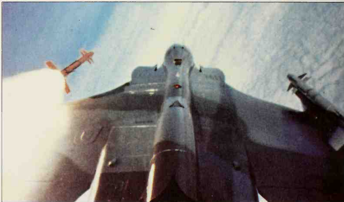
Impressive view taken by a fin-mounted camera of firing of a Matra 550 Magic dogfight missile from the left overwing launcher of a Jaguar International export version at about 20,000 ft (9000 m) in a moderate turn.
