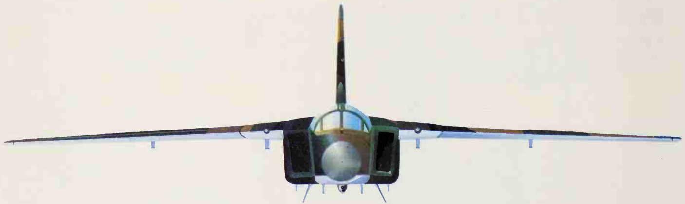
Head-on , the Su-19 closely resembles a MiG-27, and uses similar aerodynamics, but it is larger and has a wider body, broad cockpit with round-topped canopy and a nose radome. Twin ventral fins slope out
