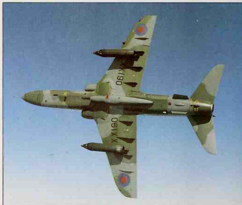
A BAe Hawk T.1 from the Tactical Weapons Unit at RAF Brawdy does a slow roll to show off its centreline 30-mm Aden gun pod and two SNEB rocket pods on the wings.
