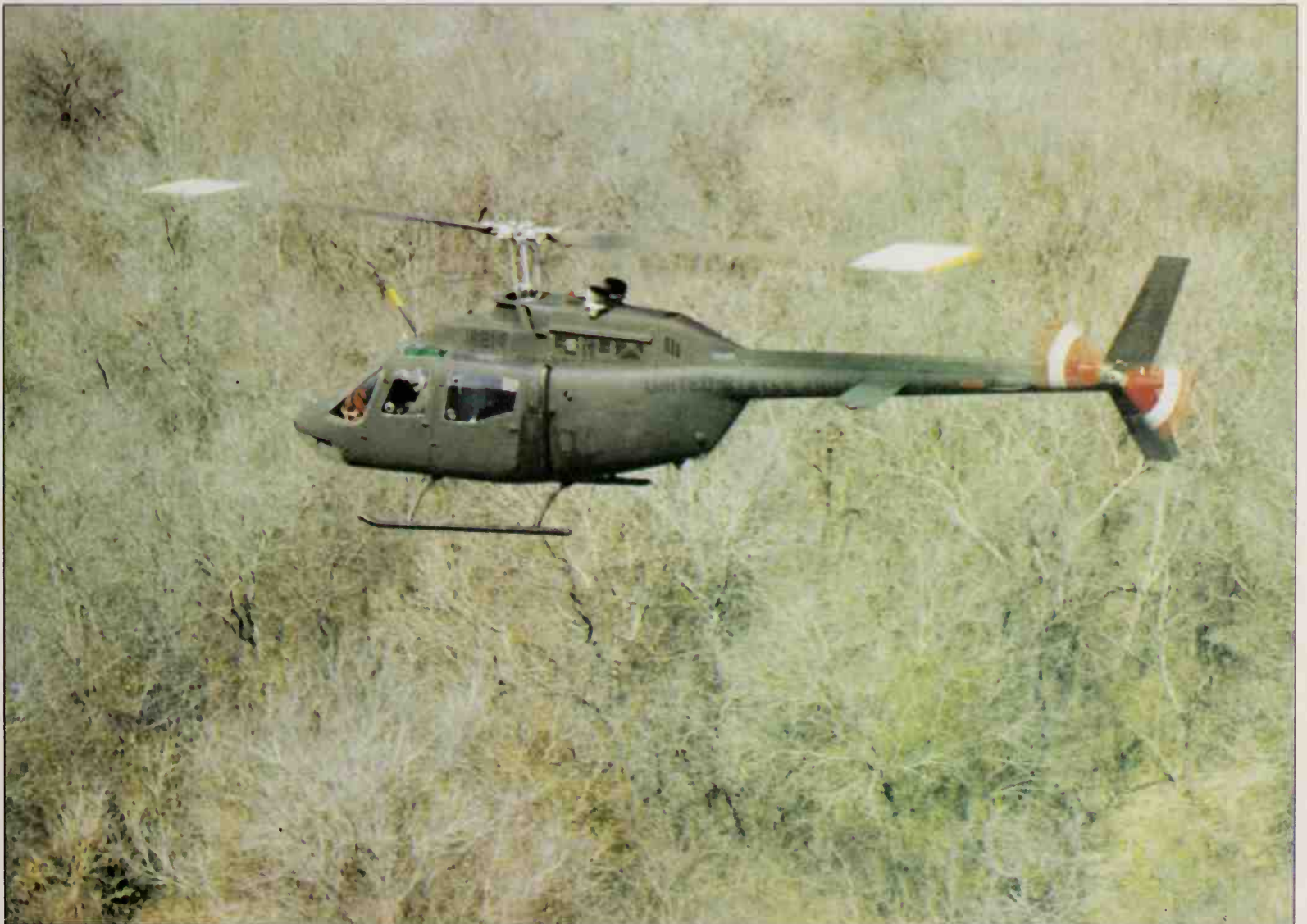
OH-58C development version of the Bell OH-58A Kiowa. This has an uprated 420-shp (313-kW) Allison T63-A-720 turboshaft engine, and a flat glass canopy to eliminate reflections. If this version enters production it is likely to introduce many improved avionics, maintenance and survivability features.
