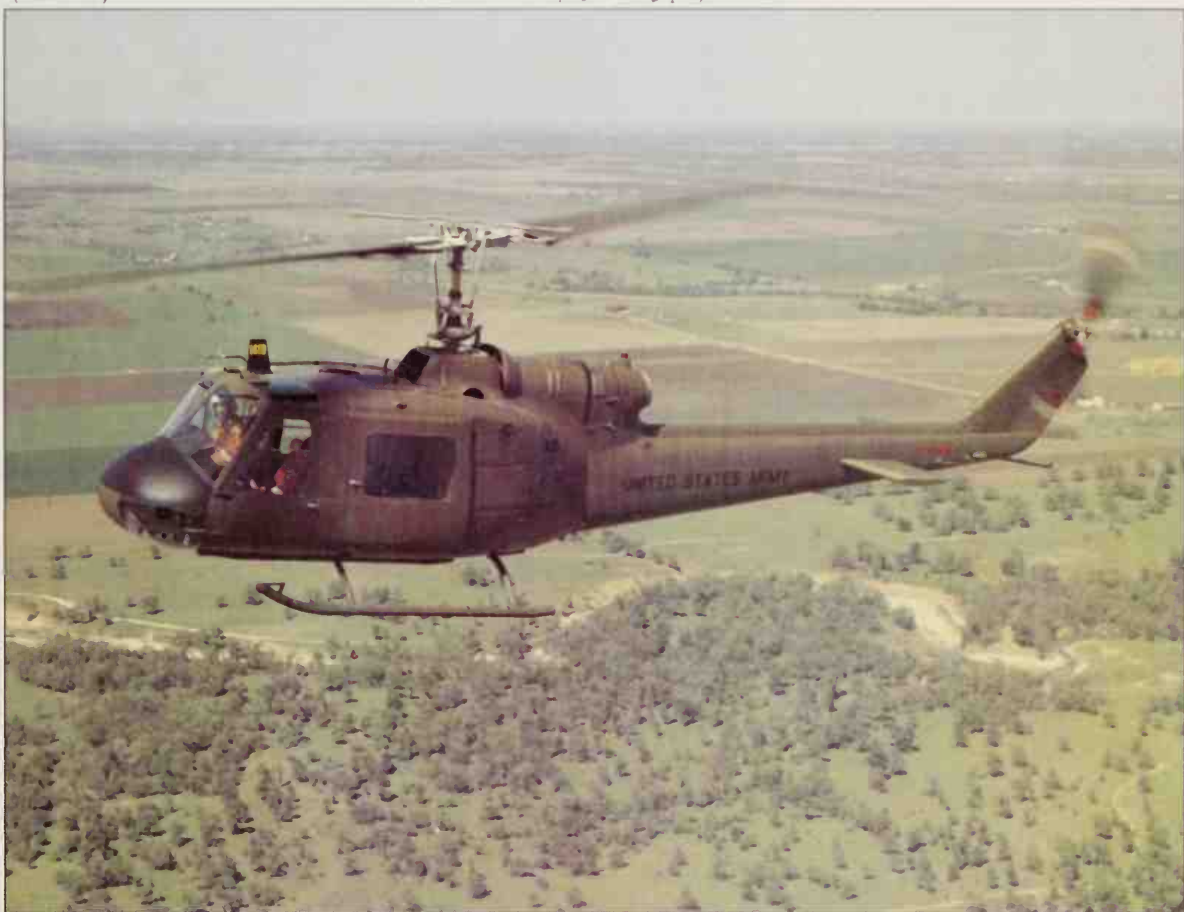
Bell Model 204/UH-1B Iroquois. The military version of the Bell Model 204 was the first turbine-powered aircraft to enter service with the US Army. UH-1Bs armed with machine-guns or rockets were deployed in a close-support role in Vietnam.
