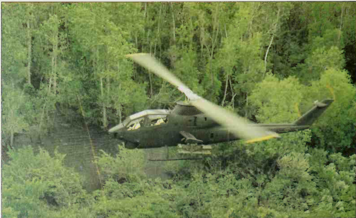
Bell single-engine Model 209 HueyCobra/AH-1S , an advanced TOW-missile equipped version of the AH-1G/Q. A distinctive feature is the flat plate canopy, designed especially to eliminate unwanted reflections.
