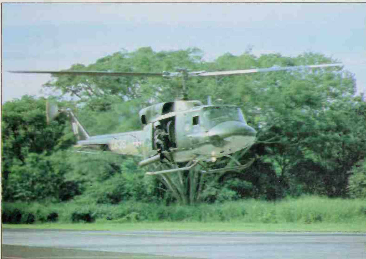
Bell UH-1N general-purpose helicopter. Modern rotary-wing aircraft in this class offer completely new standards of performance as a result of using advanced main rotors and twin-turbine powerplants. Either turbine is able to maintain safe flight if one engine fails.
