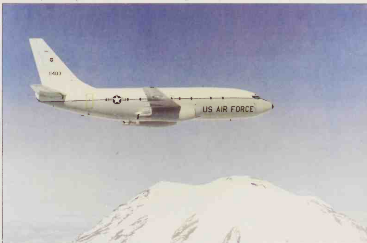
The Boeing T-43A is the chief navigation trainer of the US Air Force, a fleet of 19 operated by the 323rd Flying Training Wing at Mather AFB, California, having replaced 77 Convair T-29s. The T-43A is based on the Boeing 737-100, although with major changes.
