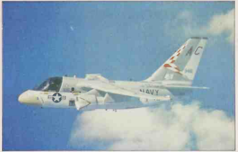
Lockheed S-3A Viking anti-submarine aircraft attached to the USS Saratoga . The four-man crew of each Viking has available the most advanced sonobuoys and MAD equipment to seek out the quieter, deeper-diving submarines which are currently in service with major powers.
