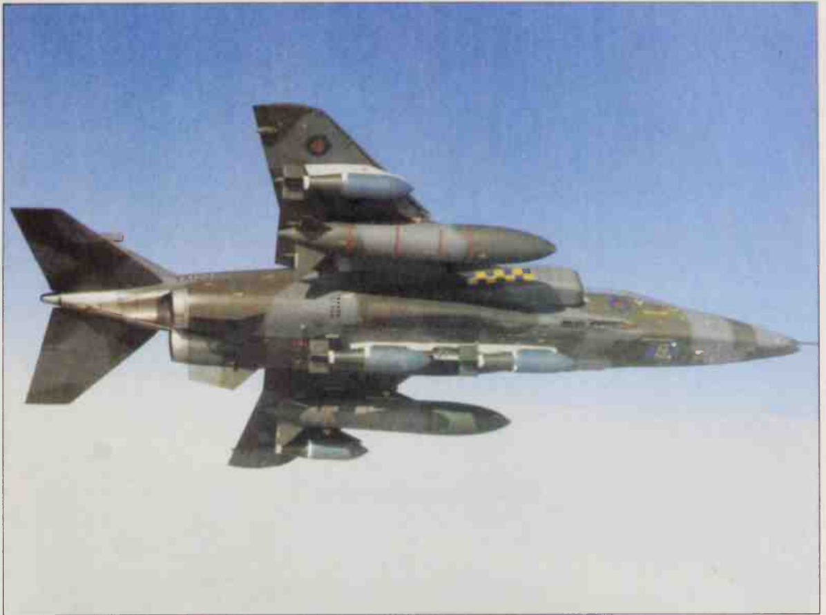
This SEPECAT Jaguar GR.1 of 54 Sqn, RAF Coltishall, has done a lot of hard flying at low level but seems rarely, if ever, to have fired its very useful twin 30 mm guns. The GP bombs are described as 500 kg, or 1,102 lb, instead of the previous "1,000 lb" continued
