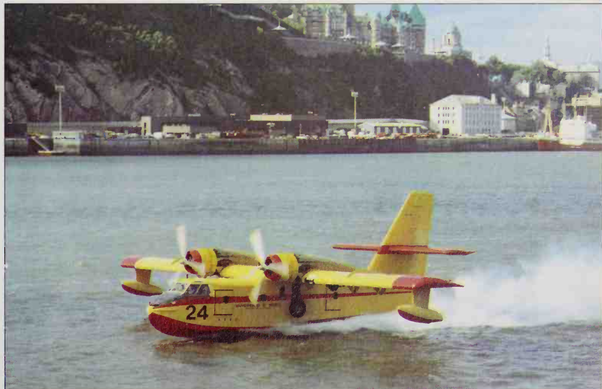
One of the Province of Quebec's Canadair CL-215 amphibians pictured on the St Lawrence river at Quebec City. Designated initially as a firefighting aeroplane, the CL-215 also serves in the search and rescue and patrol roles.
