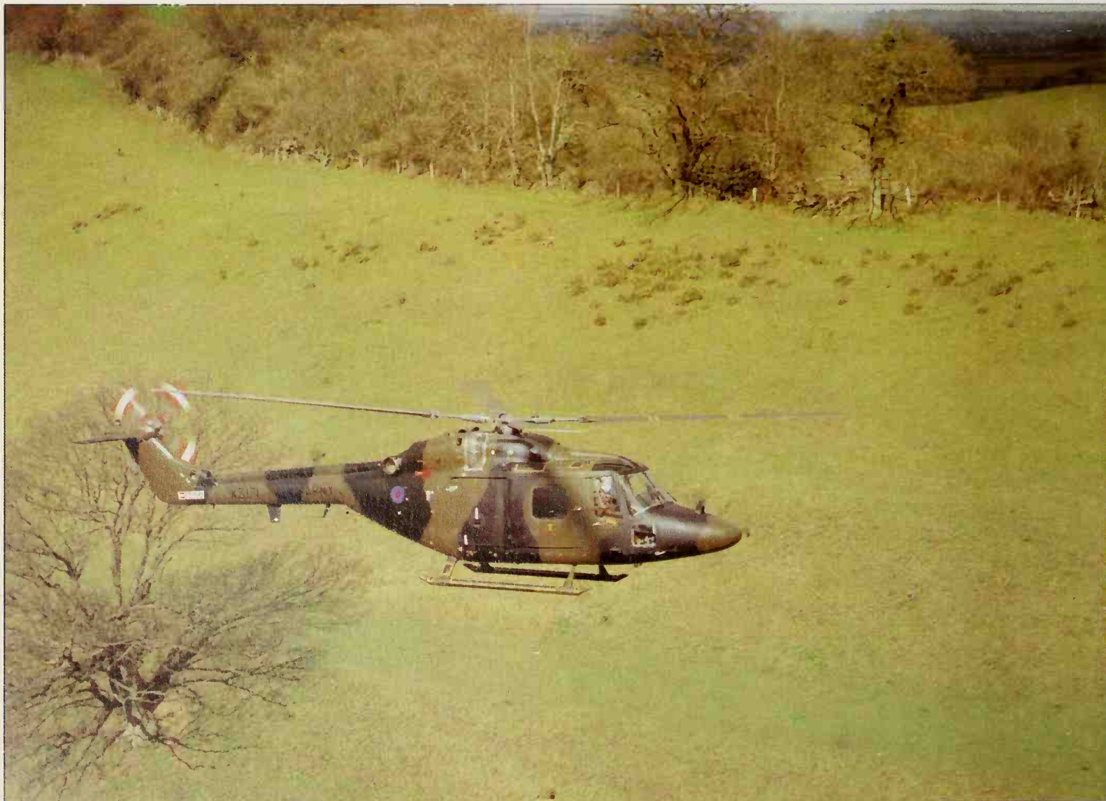
This Westland Lynx AH.1 was photographed during type conversion training with the Lynx Intensive Flying Trials Unit at Middle Wallop. This unit has since disbanded, and Lynx are building up in strength in Germany, with HOT missile sights and pylons.
