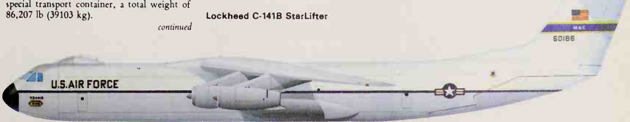
Lockheed C-141B StarLifter, prototype long-fuselage conversion of the standard C-141A, of Military Airlift Command, USAF.
