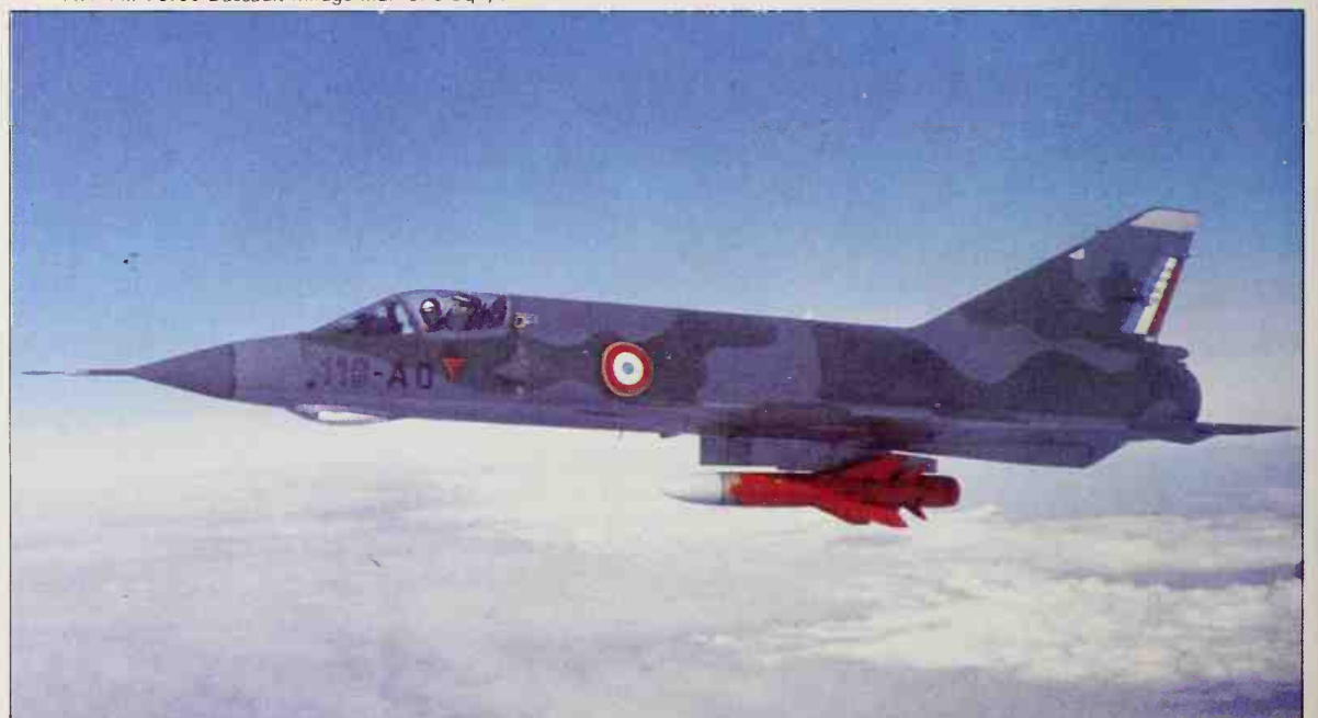
This Dassault Breguet Mirage IIIE, the 512th off the assembly line, is seen in the stand-off attack role armed with an AS.37 anti-radar Martel. France has not bought the more useful British-developed TV-guided version of this collaborative missile.
