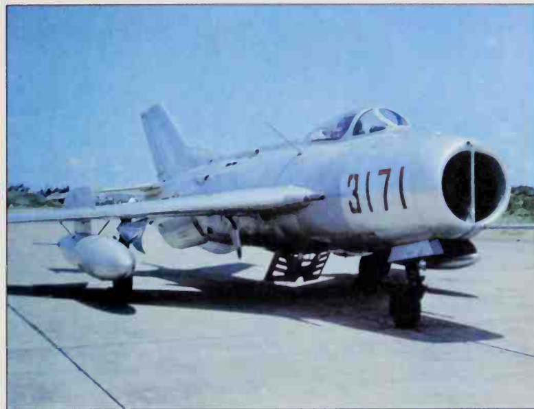
The Chinese Shenyang F-6. This type of tactical fighter/bomber has proved extremely well built and reliable, and Western observers have praised the detailed finish of the airframe. China also builds the engines and NR-30 gun.
