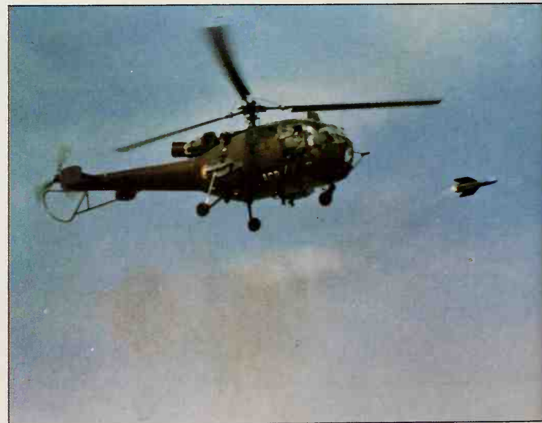
Firing an AS.11 from Alouette III, a combination widely used by the French ALAT and several other countries. Replacements for different roles include the anti-tank HOT and the anti-ship AS.15, still under development.
