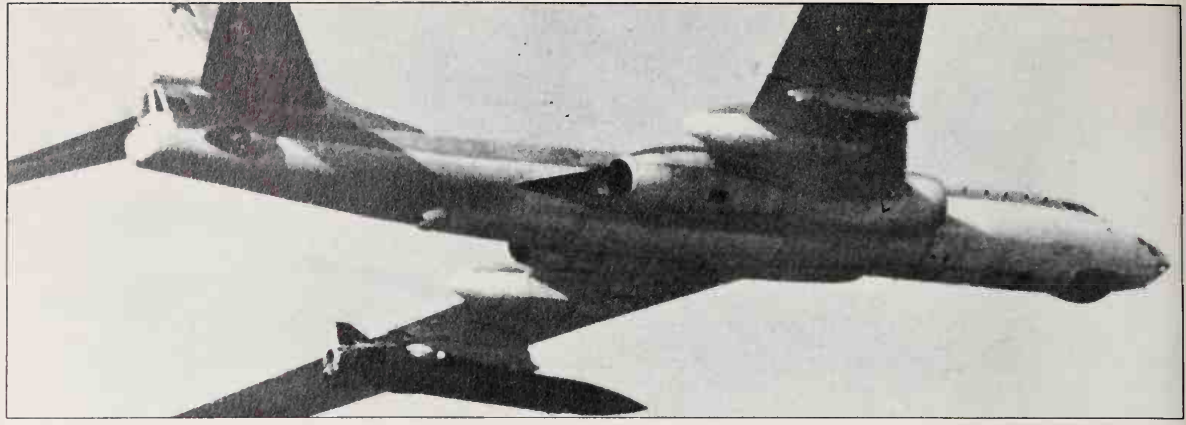
Designated AS-6 'Kingfish' by NATO, the missile under the left wing of this Tu-16 'Badger-H' is a standard weapon of the 'Backfire'.
