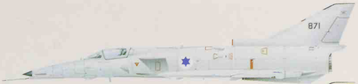
Israel Aircraft Industries Kfir-C2 in air superiority grey finish adopted for some Heyl Ha'Avir units in 1977.
