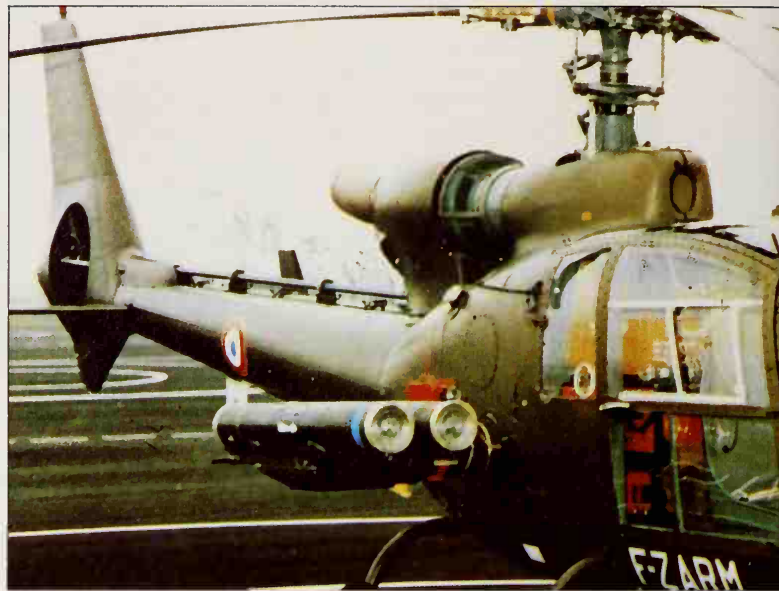
Standard new anti-tank missile of many countries including the sponsors, France and West Germany, the Euromissile HOT is seen here in a four-barrel installation on a Gazelle of the French ALAT. The German Heer (Army) BO105s carry six rounds.
