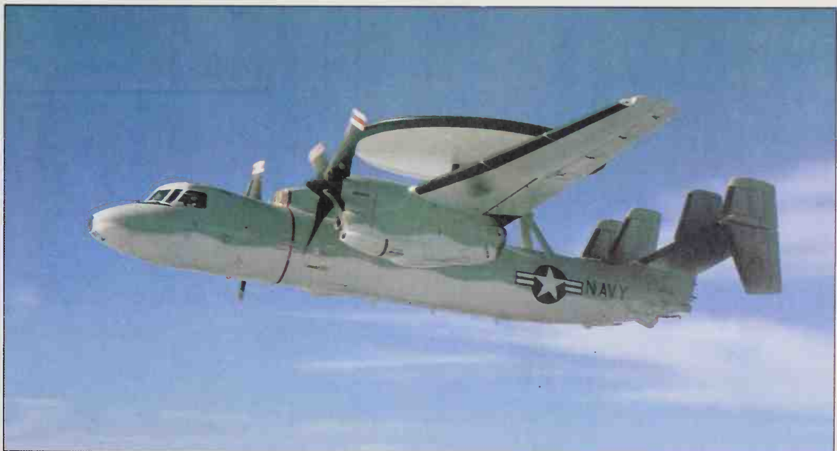
Portrait of a Hawkeye, claimed by Grumman to be more cost/effective in most scenarios than the Boeing E-3A Sentry. All versions — E-2A, E-2B, E-2C (illustrated) and TE-2C — are closely similar externally but differ greatly in electronics and systems.
