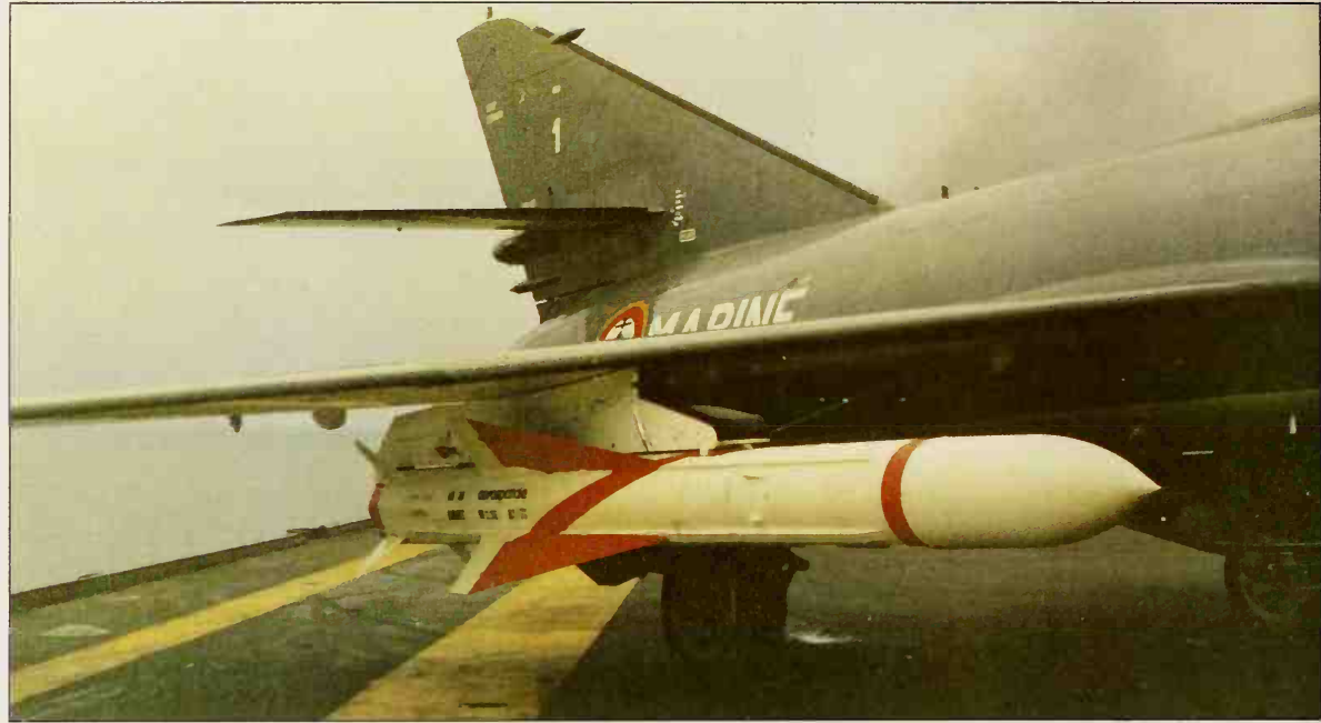
One of the carriers of AM.39 Exocet is the Super Etendard, the first prototype of which is seen here with a carry-trials AM.39 under the right wing. This large missile is also launched by the Mirage F1, Atlantic and Super Frelon.
