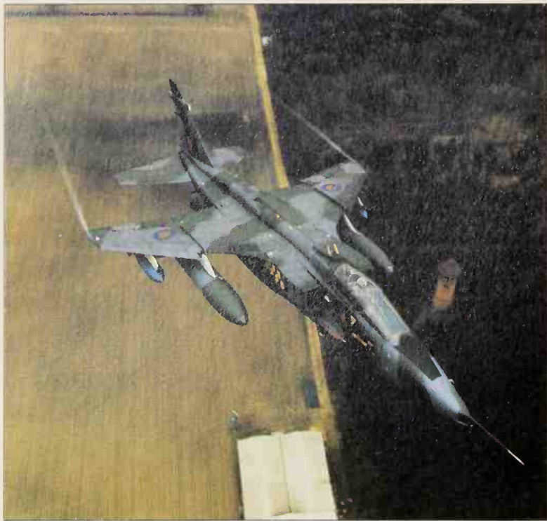
A GR.1 Jaguar from 54 Squadron, based at RAF Coltishall, carrying two 1200 litre fuel tanks and four 1000 lb bombs.
