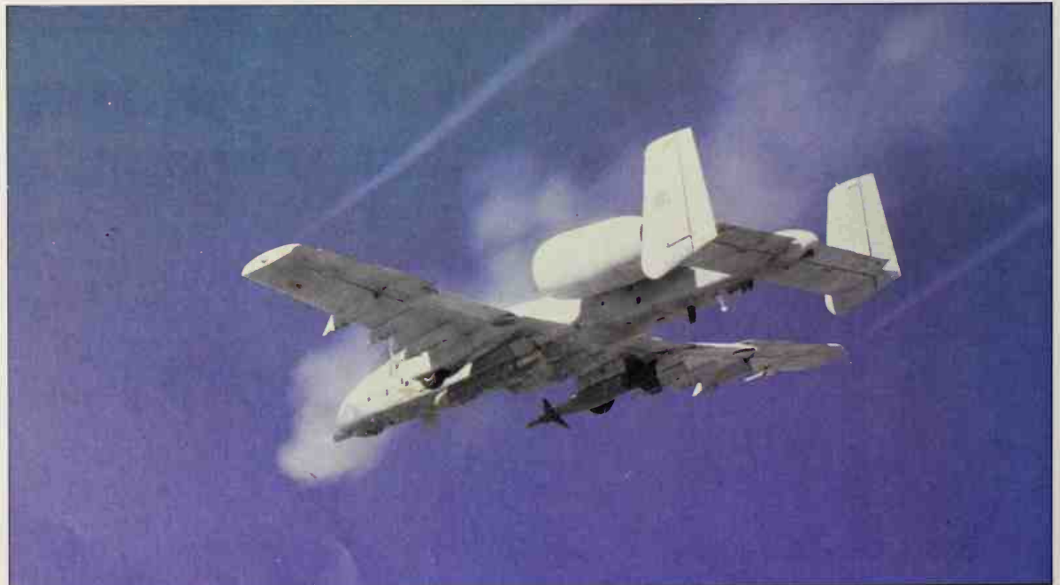
This A-10A was photographed while firing its extremely powerful tank-killing gun. One of the 11 pylons is carrying a laser-guided 'smart bomb'
