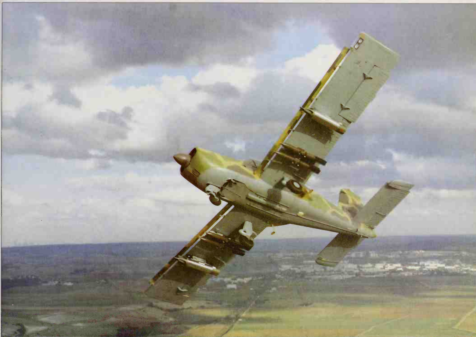
The Rallye 235G is the world's most warlike single-engined lightplane, as this four-pylon specimen emphasizes. Built by Socata, a subsidiary of France's Aérospatiale, the manoeuvrable Rallye is normally a four-seater but can swap seats for stores
