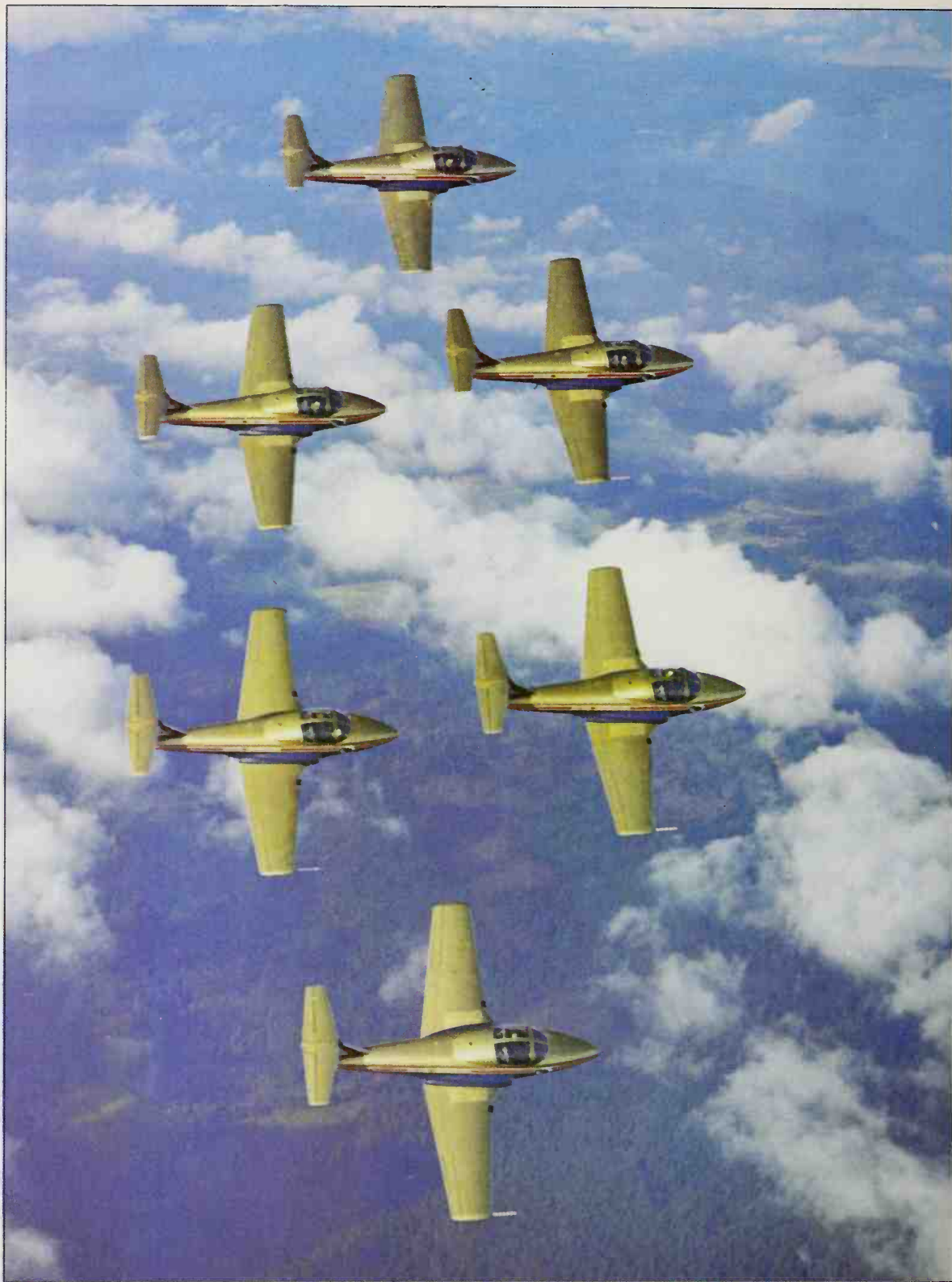
The Canadair CL-41 Tutor, called CT-114 by the Canadian Armed Forces, has equipped several CAF display teams as well as serving as standard pilot trainer to 'wings' standard at Moose Jaw. Over 100 are being updated in both structure and systems.
