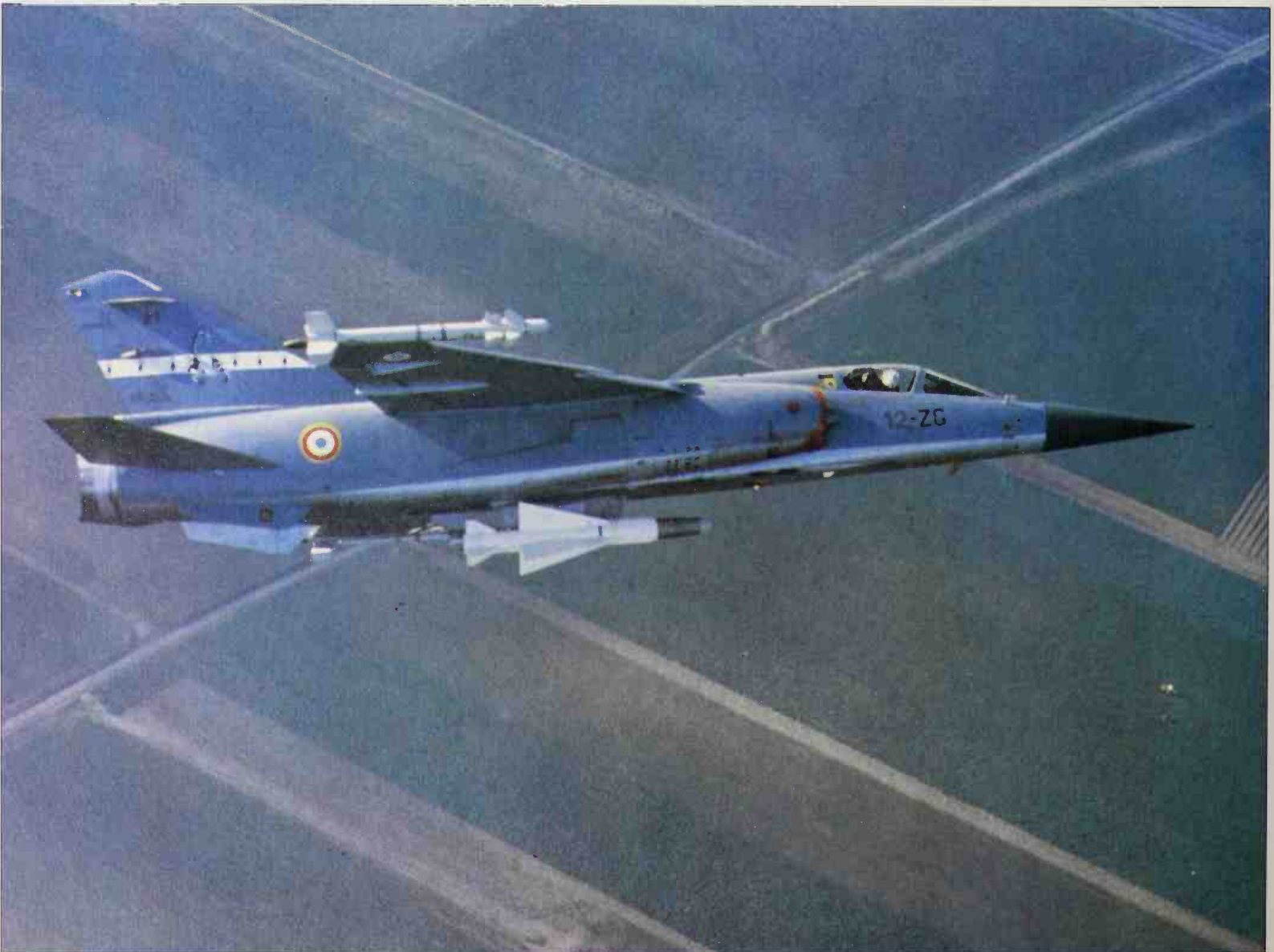
The Dassault-Breguet Mirage F1-C is the standard interceptor of the French Armée de l'Air . This, the 21st off the line, is serving with 12 ème Escadre de Chasse at Cambrai; it is toting a Matra R 530 air-to-air missile and two much better Magics.
