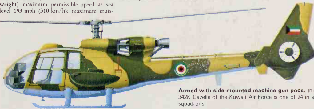
Aérospatiale SA.342 Gazelle with 'Fenestron' shrouded fan anti-torque tail rotor.
