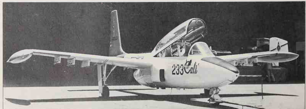
Originally called the TT-1 Pinto, this neat primary jet trainer has reappeared as the T-610 Cali, which the Self-Reliance Wing of the Philippines Air Force hopes to put into production as an armed COIN attack platform (note pylons) and trainer.
