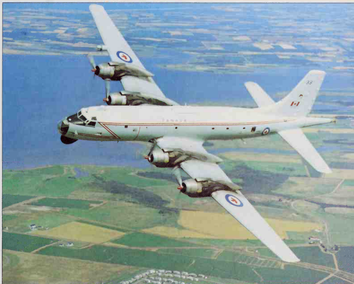
Canadair based the CL-28 Argus ASW and ocean patrol aircraft on the Britannia, although differences were so great the advantages were problematical. Called CP 107 by the CAF, these long-endurance platforms are soon to be replaced by the smaller CP 140 Aurora
