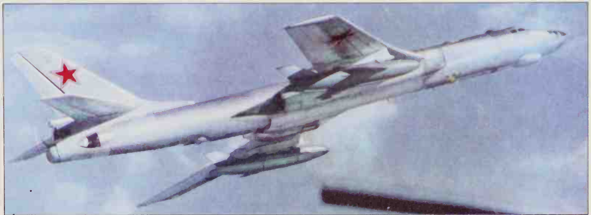
Two AS-5 'Kelt' rocket-powered cruise missiles are carried by the 'Badger-G' version of the widely used Tu-16 strategic platform
