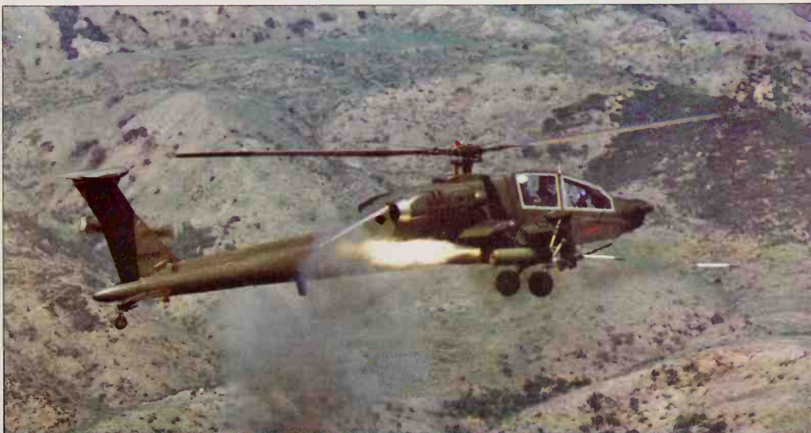
This prototype Hughes YAH-64 advanced attack helicopter is firing unguided rockets, but the primary anti-tank weapon of the production AH-64A is expected to be the precision-guided Hellfire. A total of 536 is expected to be ordered.
