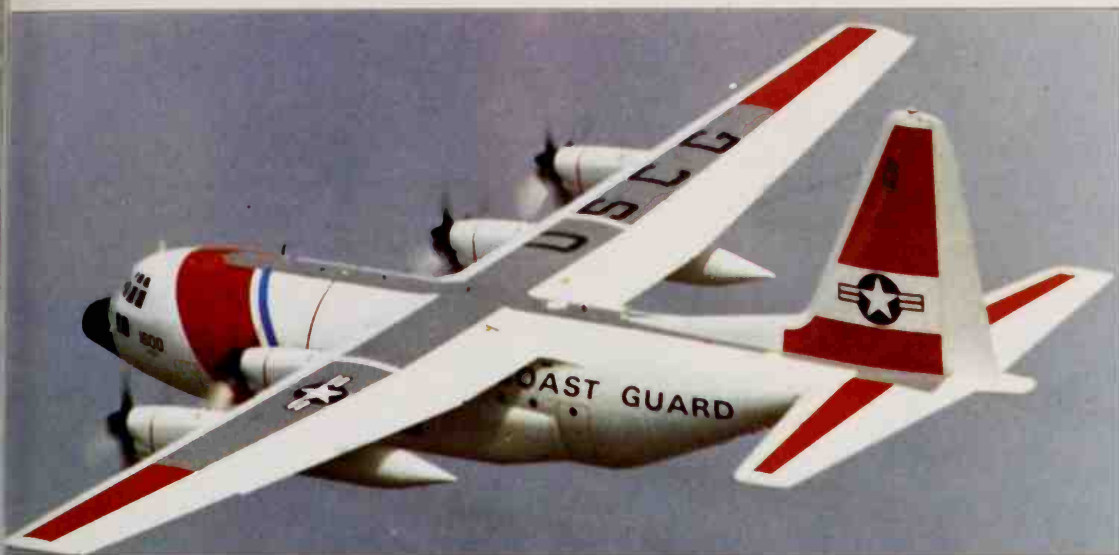
Lockheed HC-130H Hercules air search, rescue and recovery aircraft; seven examples are in service with the US Coast Guard. These have a nose-mounted recovery system able to pick up from the ground persons, or objects weighing up to 500 lb (227 kg).
