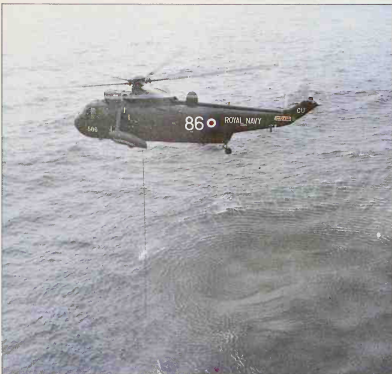
Though the transducer is not visible here the dunking sonar of this Royal Navy Sea King is probably a Plessey Type 195, which is also used by other navies
