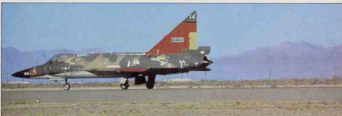
This GD (Convair) F-102 Delta Dagger is not parked on the duty runway, it has just opened up for takeoff, despite the empty cockpit. It is a Sperry/Fairchild POM-102A used in threat evaluation and other hazardous missions, flown by a remote pilot
