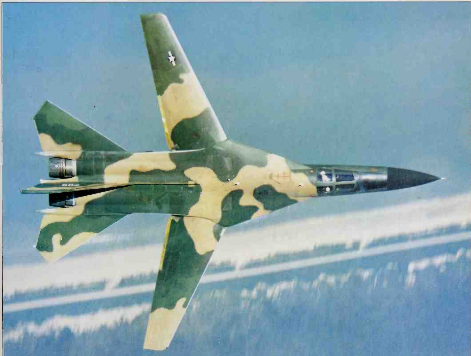
One of the first General Dynamics F-111A swing-wing attack aircraft, flying in the loiter mode with wings at 16° sweep. Violent Congressional arguments centred around the decision to procure this slightly disappointing initial version in quantity; the final F-111F is a vast improvement but only 106 could be afforded.
