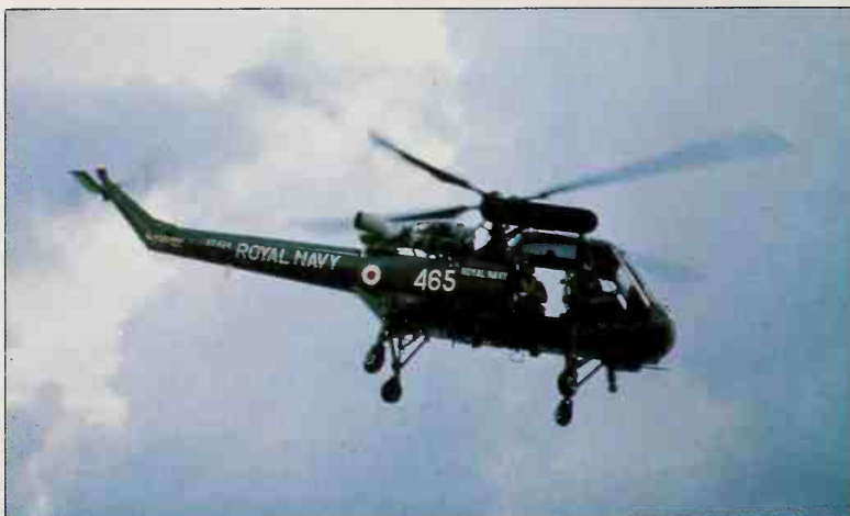
This Westland Wasp HAS.1 of the Fleet Air Arm must be draughty with both main doors wide open. It probably belongs to No 829 Sqn, which supplies the aircraft for all Royal Navy frigates. Most Wasps can carry Mk 44 or 46 torpedoes and a few have AS.11s.
