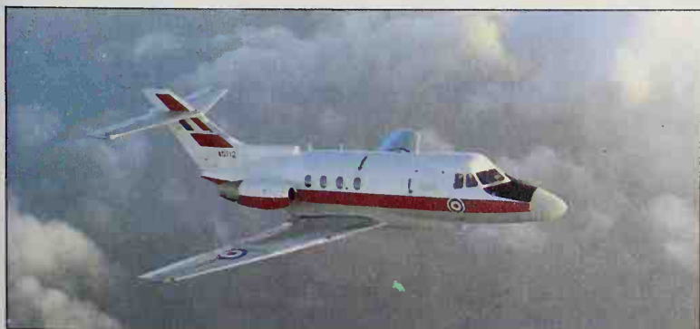
Distinguished by its bulged belly housing Decca doppler radar, and a bright red fuselage stripe, the Dominie T.1 equips 6 FTS at Finningley where the RAF's navigation training is centred. Some 19 are in use.
