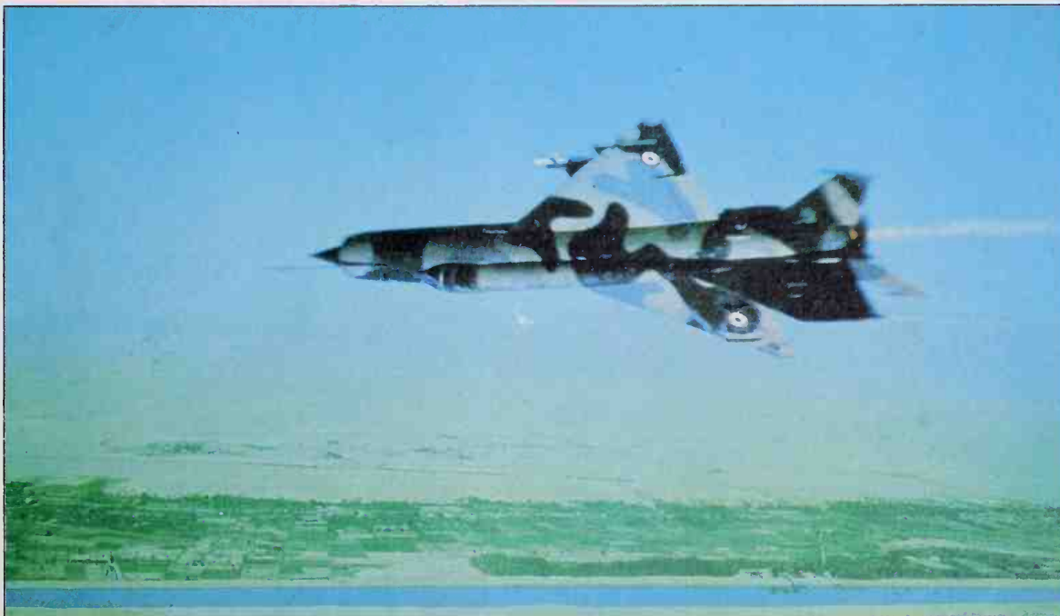
Long one of the world's largest users of Soviet equipment, the Egyptian AF appears still to be in receipt of such arms as witness this very new MiG-21bis (the current model with a new airframe including a large dorsal spine).
