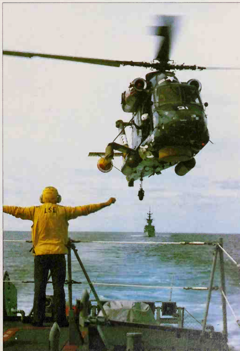
Kaman's SH-2F Seasprite is a vastly more capable helicopter than the original single-engined Seasprites, and has for a decade been the "Interim LAMPS" platform for US Navy frigates and other ships, with radar, sonics, MAD bird and torpedoes.
