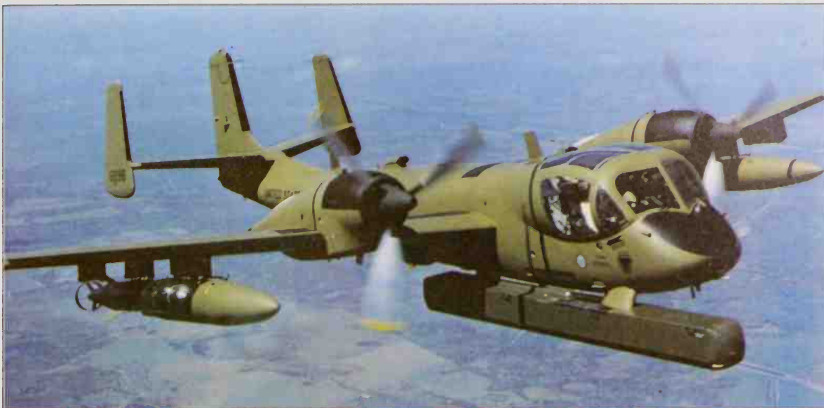
The Grumman OV-1 Mohawk is a unique STOL platform for carrying sensors over land battlefields. This US Army OV-1D is burdened with APS-94 SLAR (side-looking airborne radar), tanks and bombs. Many have been converted to serve as EW/Elint aircraft.
