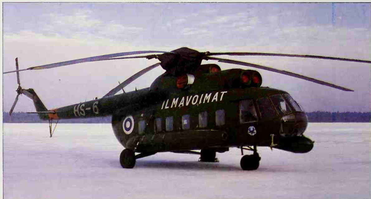
Six Mil Mi-8P passenger helicopters, with the large windows of the civil version, form the chief rotary-wing transport element of Finland's Ilmavoimat. Since delivery they have been equipped with weather radar under the nose.
