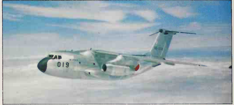
A production Kawasaki C-1 of the Japanese Air Self-Defence Force. Although very limited in payload and range, this twin-JT8D aircraft is being updated gradually, and the final batch have a centre-section tank added. Total deliveries by 1980 are to be 28.
