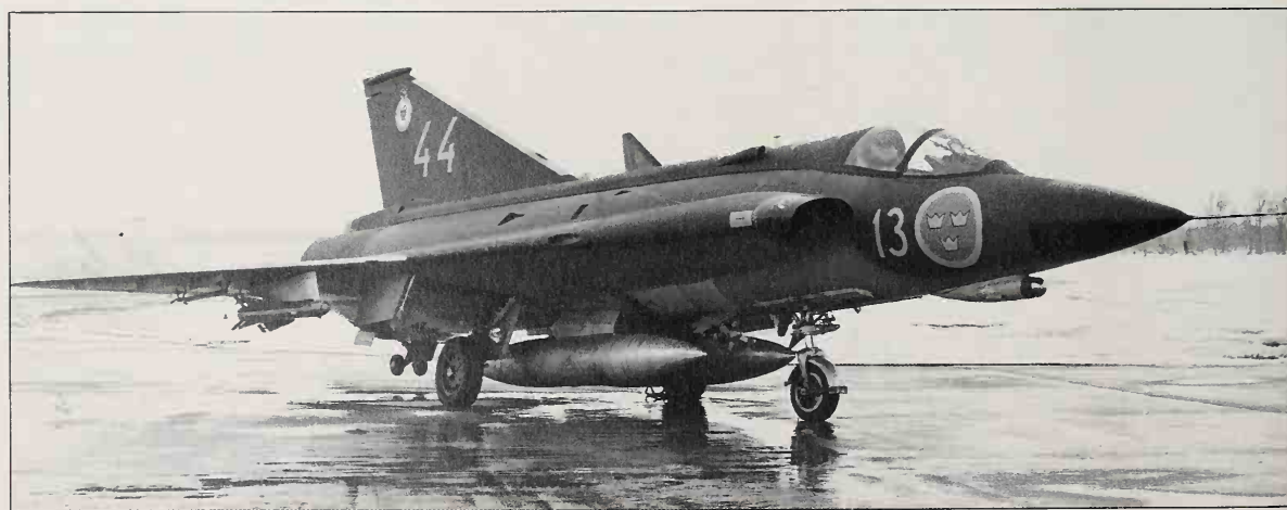
J35F 'Filip' of the Swedish Flygvapen , with a Hughes-developed weapon system including an advanced radar (made by Ericsson), IR sensor (seen under the nose) and Swedish-made Falcon missiles.
