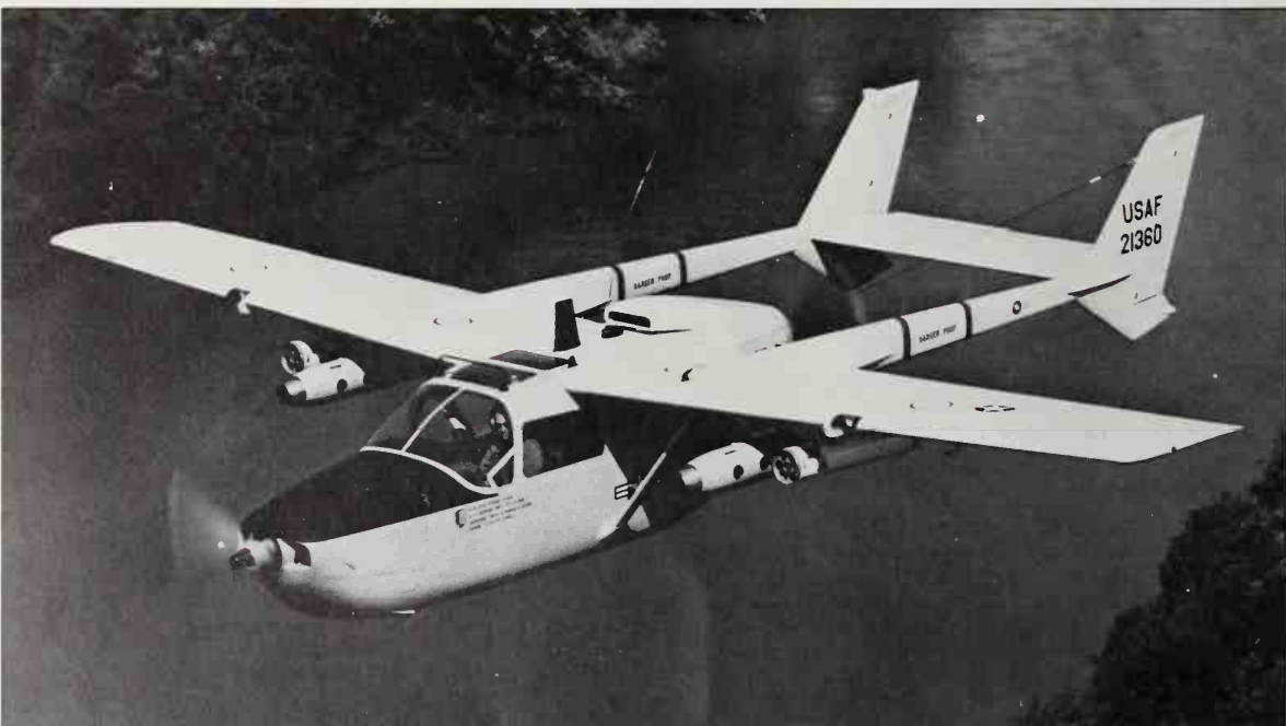
The unusual Cessna O-2 series, with push/pull engines derived from the Skymaster, was the chief lightplane FAC (forward air control) platform in Vietnam. By 1969 the USAF had 346 of the multi-role O-2A, illustrated, plus 164 'psy-war' O-2B aircraft.
