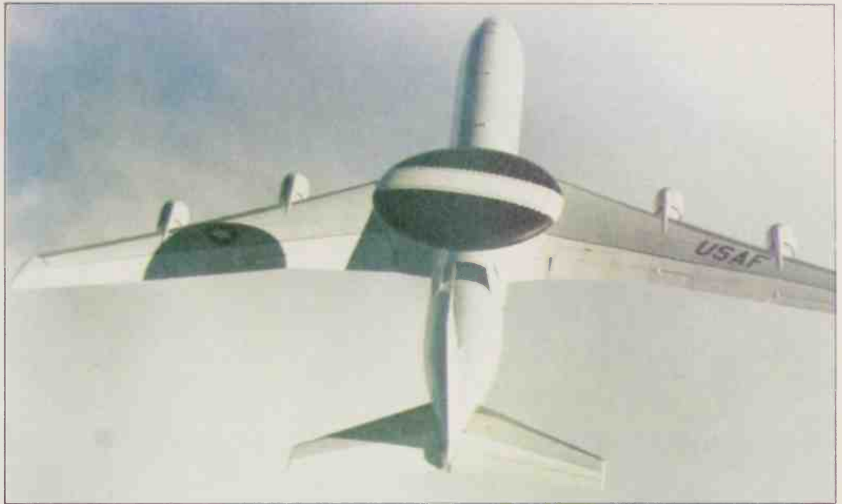
The easily identifiable Boeing E-3A Sentry Airborne Warning and Control System (AWACS) aircraft for service with the USAF. The 30-ft (9.14-m) diameter rotodome houses a 24-ft (7.32-m) diameter antenna
