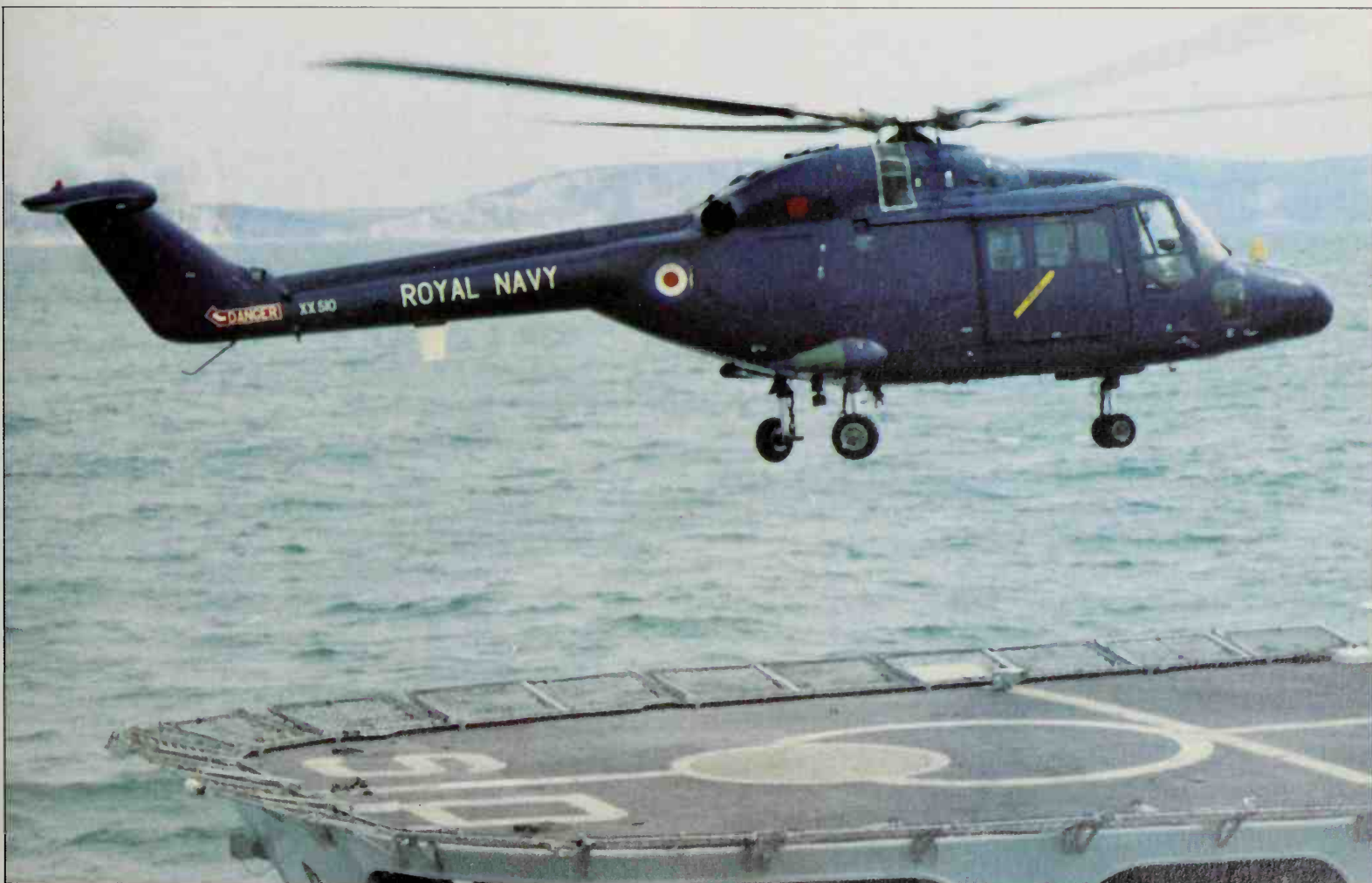
Unquestionably the most important new multi-role military helicopter, already adopted by 13 countries, the Westland-Aérospatiale Lynx is seen here in its naval version with wheel landing gear, nose radar and extensive mission equipment. This is a Lynx HAS.2 of Royal Navy 702 Sqn, probably over the fantail pad of HMS Sheffield.
