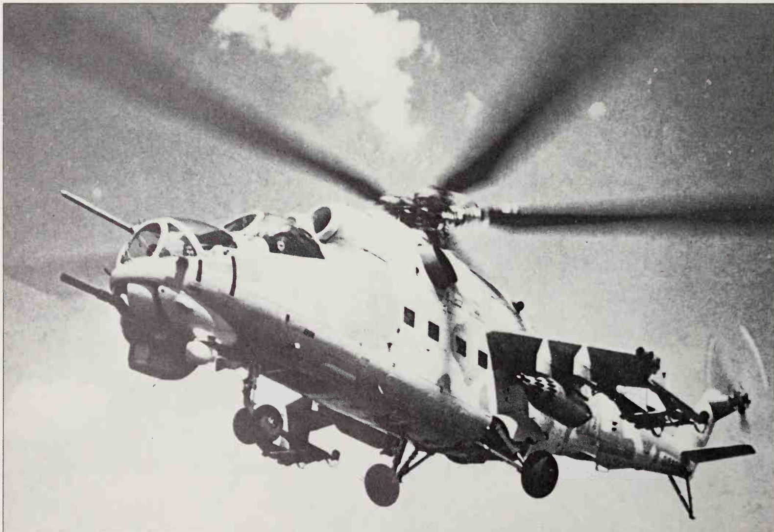
Serving in large numbers with the Soviet 16th Air Army, part of the GSFG (Group of Soviet Forces in Germany) the 'Hind-D' is a multi-role attack helicopter of formidable capabilities. Now believed to be designated Mi-27, it has eight weapon pylons, a 'Gatling' cannon and a comprehensive array of avionics and sensors. The long pole in the nose is a low-air-speed sensor.
