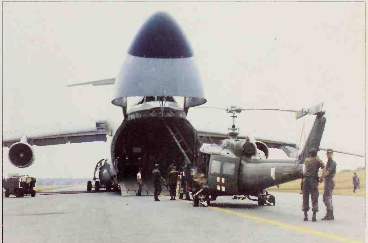
This illustration of the Lockheed C-5A Galaxy gives some scale to the size of this very large transport aircraft. With the visor type nose door raised, a Bell UH-1 Iroquois helicopter, itself almost 42 ft (12.80 m) long, can be loaded without difficulty.
