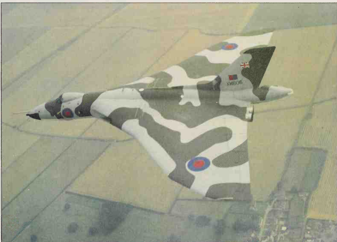
The British Aerospace Vulcan B.2 is another long-serving type which has been continually updated, some of the electronics changes showing externally. The RAF also has four rebuilt as SR.2 strategic reconnaissance platforms, serving with No 27 Sqn at Scampton.
