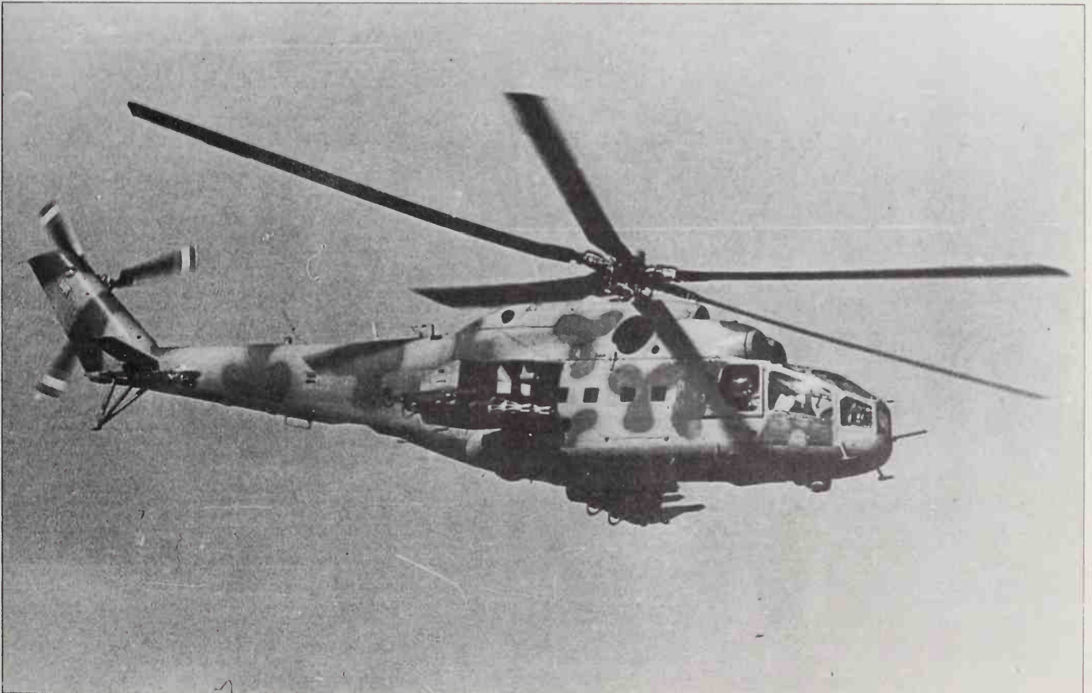
One of the latest and best photographs of the Mil Mi-24 version known as 'Hind-A' to NATO, this appears to show a six-bladed main rotor, though this may be an illusion caused by the upward flexure of the blades. Since 1974 possibly 1,000 of several versions of these versatile machines have entered Soviet service.
