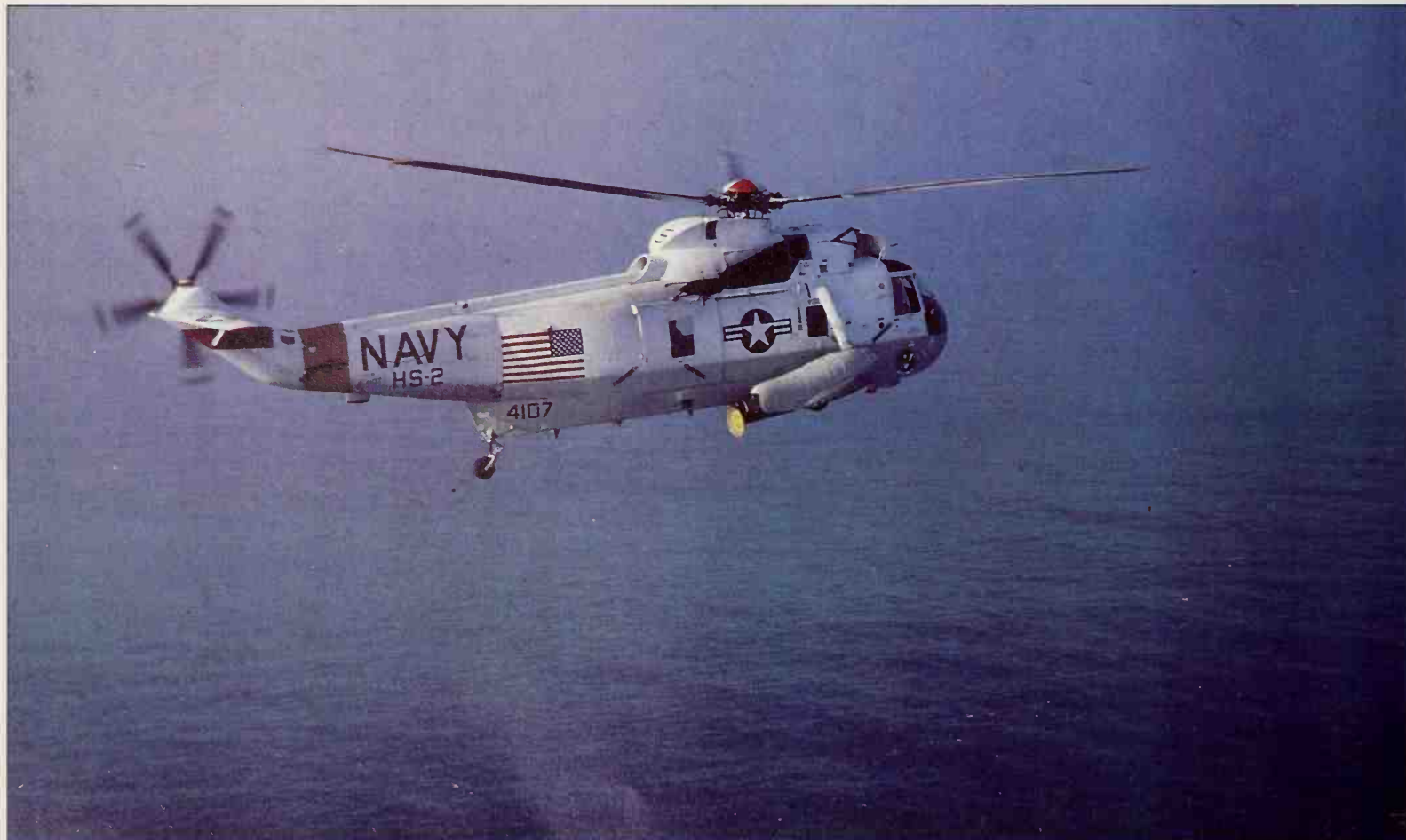
This Sikorsky SH-3D Sea King, of US Navy squadron HS-2, is one of about 80 serving with ten ASW squadrons. Some ASW Sea Kings have been rebuilt to SH-3G and -3H utility and multi-purpose configuration, and the Sikorsky SH-60B will soon arrive.
