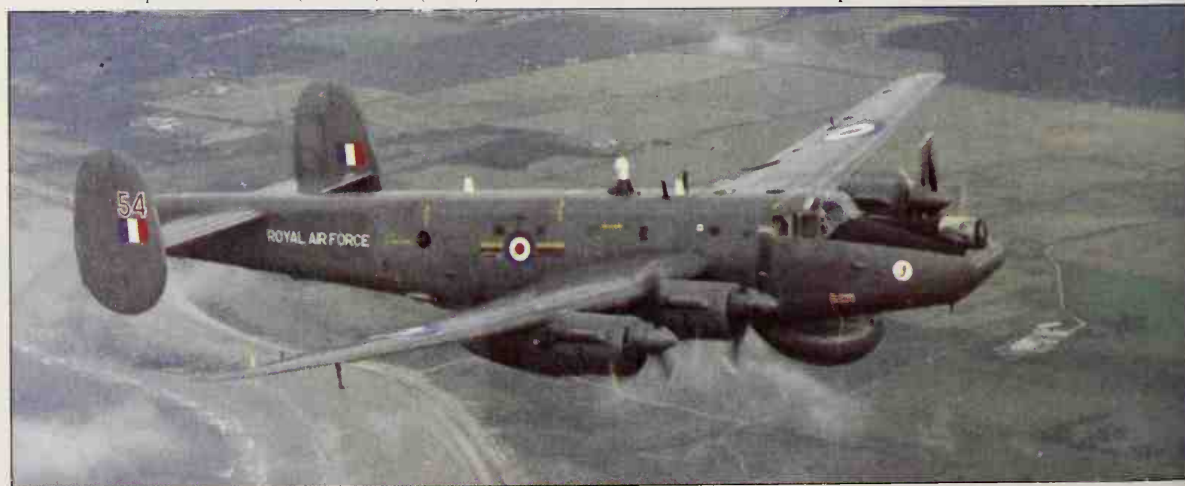
An airborne early-warning Shackleton, WL 754 of No 8 Sqn, RAF, going out on patrol from Lossiemouth in August 1977. The Shackleton AEW 2 was a rebuild of an outdated MR patrol platform with a 'third-hand' radar previously used in the AD-4W and Gannet.
