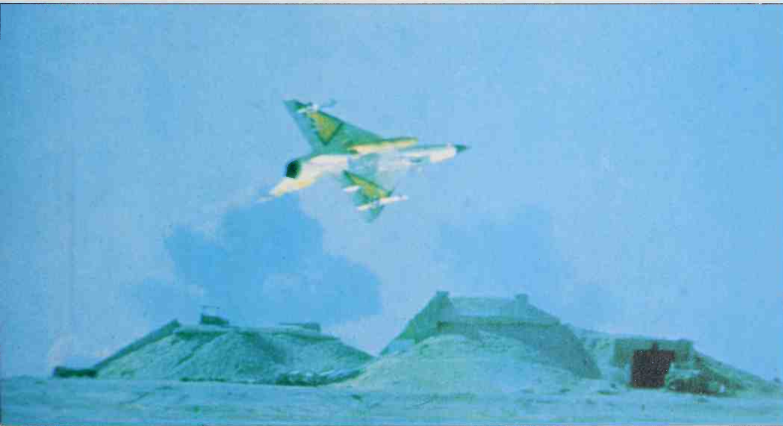
Though its canards are not clearly visible, this flamboyantly demonstrated IAI Kfir is probably one of the standard C2 production models, carrying what appear to be two Shafir AAMs and the largest size (1700-litre, 374 Imp gal) centreline drop tank. Buildings in the background are hardened against air attack.
