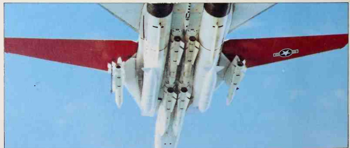
Six Phoenix AAMs are seldom carried at once by F-14A Tomcats on inventory duty, but this photograph was taken during the AIM-15A development programme. Current AIM-54B missiles have cheaper sheet-metal wings and fins, and part-digital guidance.
