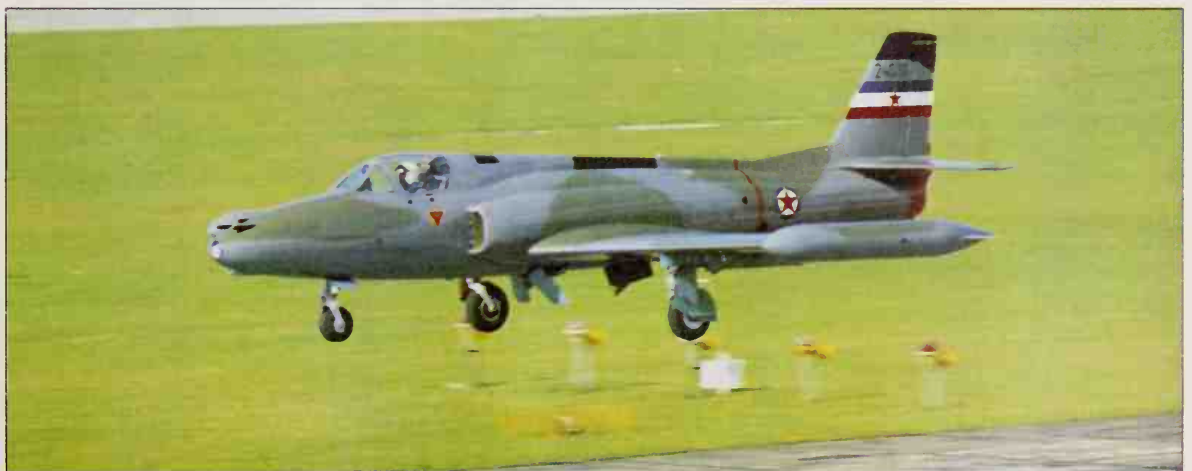
The locally built Soko Jastreb is the chief Yugoslav ground-attack aircraft, though it is planned to be replaced eventually by the Yugoslav/Romanian Orao; powered by a Rolls-Royce Viper, it is based on the Jastreb trainer.
