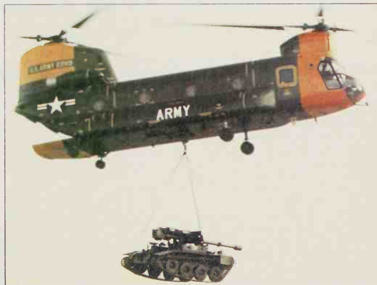
The US Army has over 620 Chinook heavy-lift helicopters, one of which is seen here with rear doors open and an old M56 Scorpion slung underneath as a test load. The US Army hopes to have most Chinooks rebuilt by Boeing Vertol to advanced CH-47D standard.
