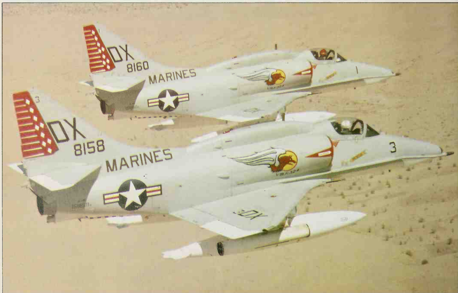
McDonnell Douglas A-4M Skyhawk II single-seat attack bomber, in production until 1979 for the US Marine Corps. It is equipped as standard with a braking parachute which makes it possible to deploy this aircraft operationally from fields only 4,000 ft (1,220 m) in length.
