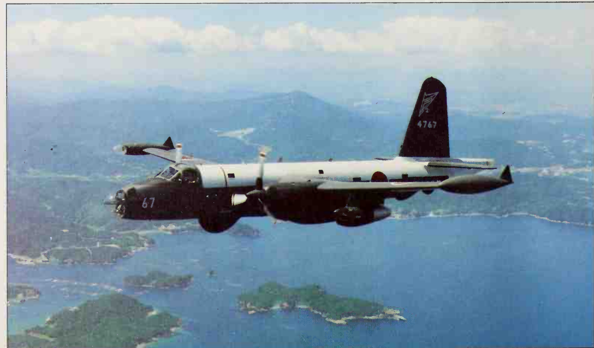
A Kawasaki P-2J of the Japanese Maritime Self-Defence Force's 2nd Koku-gun , based at Hachinoe, is pictured on patrol. This derivative of the Lockheed P-2 Neptune is the principal Japanese long-range maritime patrol aircraft, serving with four front-line units in this role.
