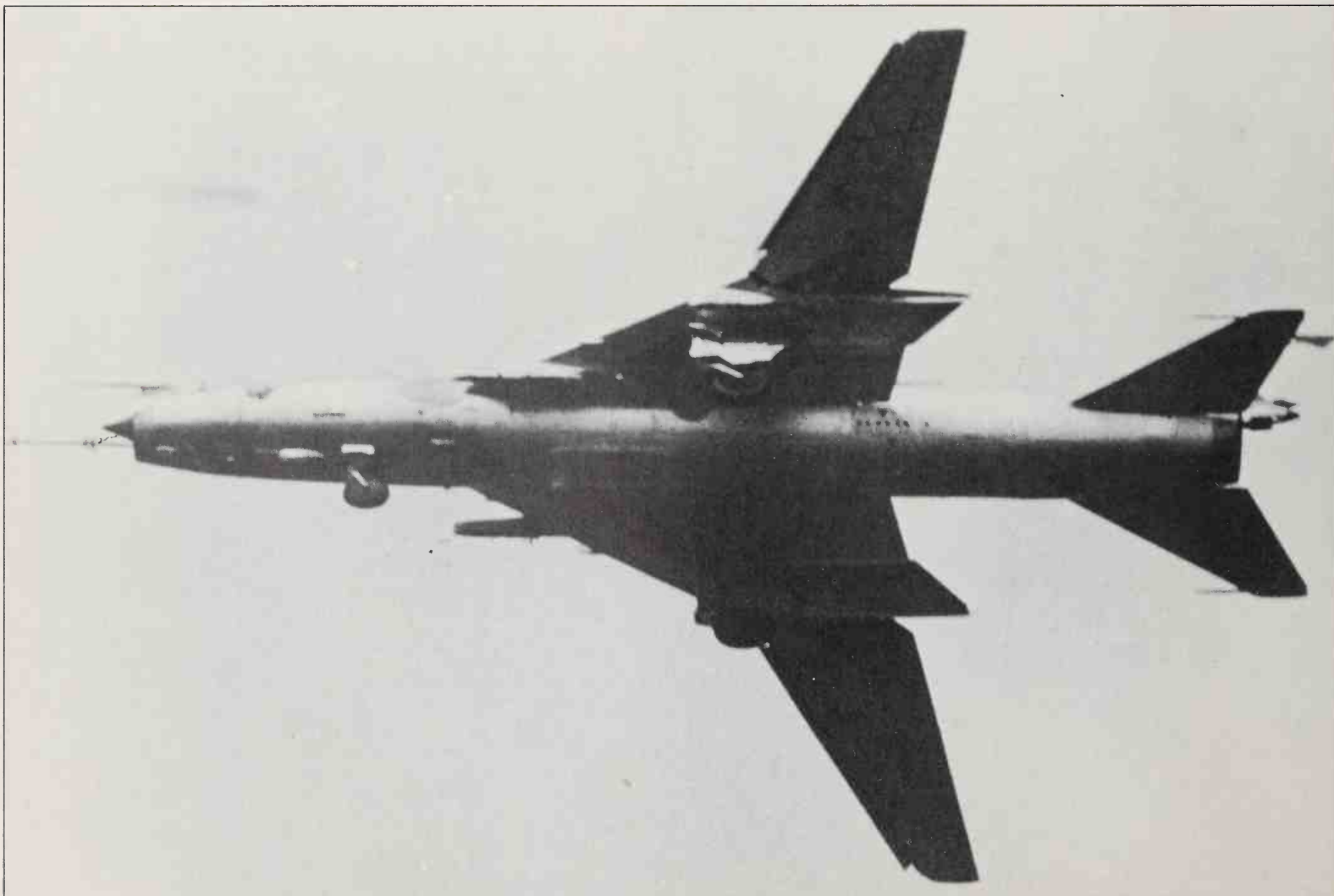
The swing-wing Su-17 is a vast improvement over the fixed-sweep Su-7 series, but still a basically old and limited design. This Frontal Aviation example is a common 'Fitter-C', but there are several other versions, some better and some (export) worse.
