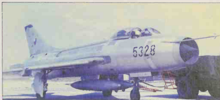
Now ready for retirement from operational service, though still available as a fuel-hungry trainer, the early Su-7B is still in wide use as a close-support and attack platform with the Czech CL. This one is starting the AL-7F engine.
