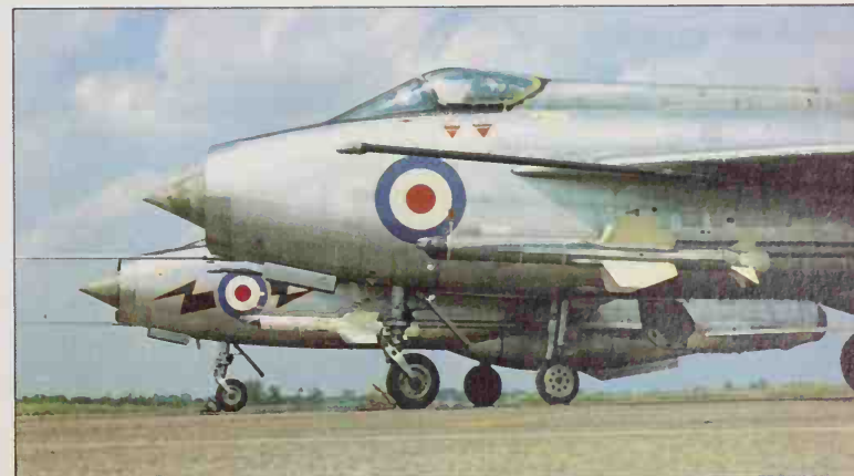
Red Top, carried by the nearer of these early Lightning interceptors, was the improved IR-homing air-to-air missile that replaced Firestreak (carried by the more distant aircraft) in RAF service. Red Top remains in use at RAF Binbrook.
