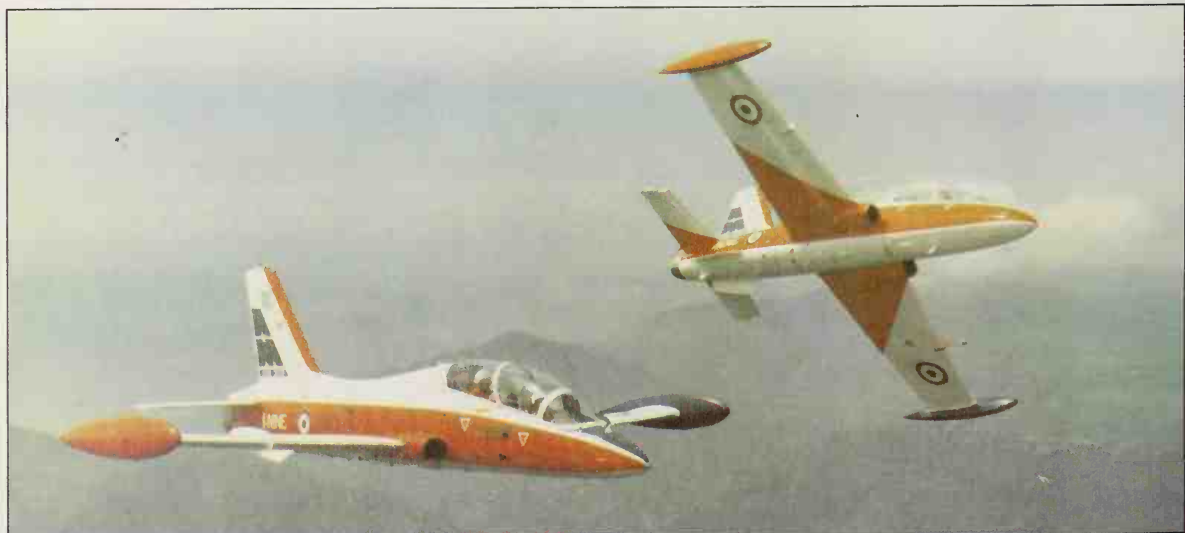
First (on the right) and second prototypes of the Aermacchi M.B.339, the improved and updated successor to the M.B.326. The first of an initial batch of 15 production aircraft for the Aeronautica Militare flew in 1978, and 100 in all are on order.
