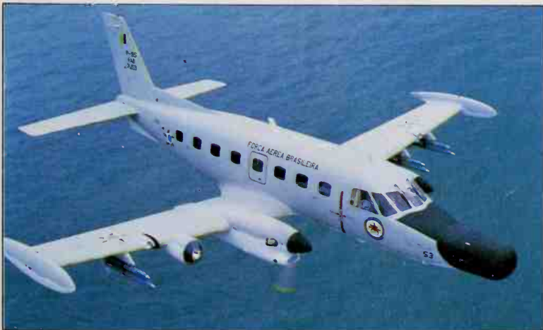
Brazil's FAB 7º Grupo uses the P-95, FAB designation of the EMBRAER EMB-111 offshore patrol aircraft. This twin-turboprop product of the world's sixth-largest aircraft company has APS-128 nose radar, Litton inertial navigation system and searchlight.
