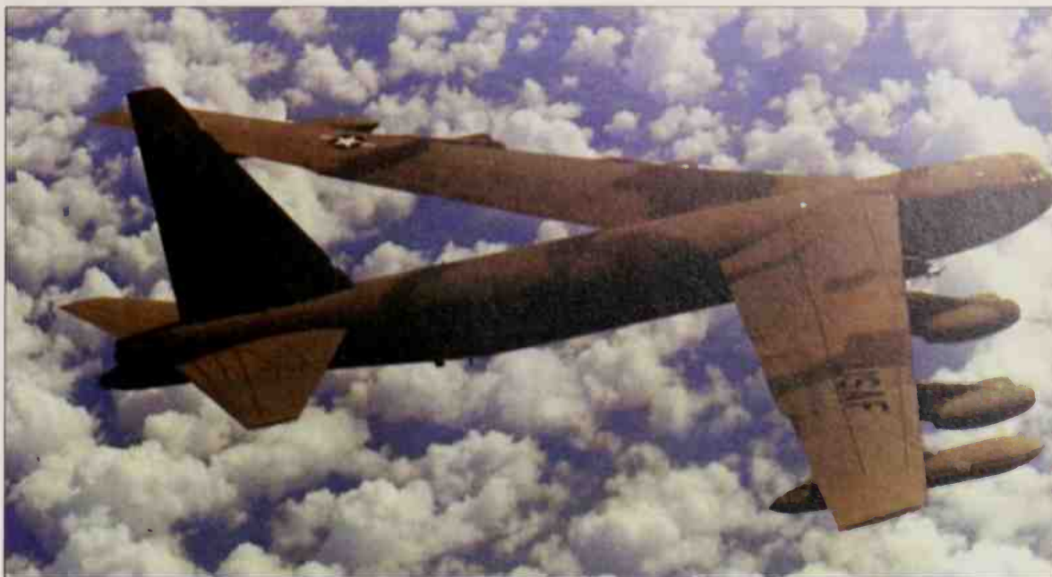
This B-52D, originally aircraft 56-581 but repainted 0-60581 in red on the new camouflage and black scheme for changed circumstances, was photographed during early 'Arc Light' bombing missions over Vietnam in 1966. It has the Big Belly structural rebuild
