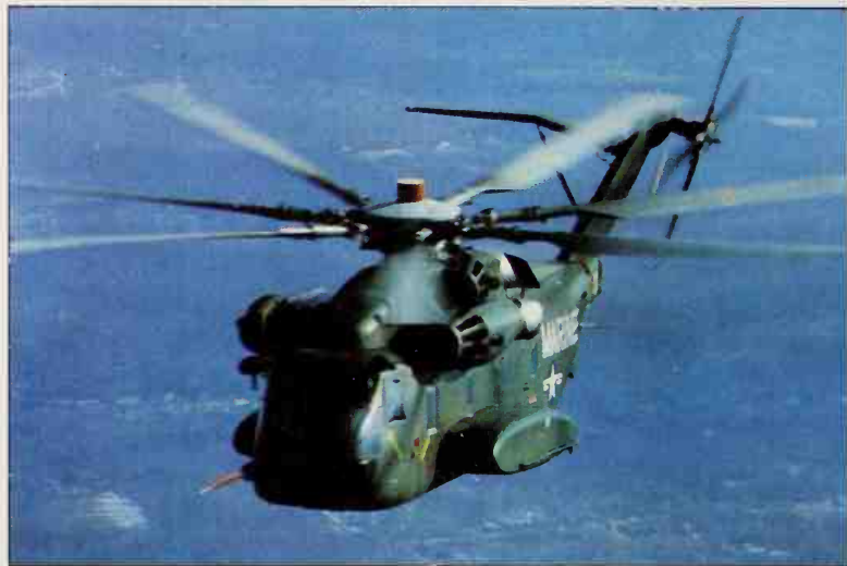
The Sikorsky YCH-53E, prototype of the new three-engined S-65 family, is in many ways the greatest helicopter in the Western skies, with 13,140 hp (9802 kW) compared with the 5,700 hp (4252 kW) of most versions.
