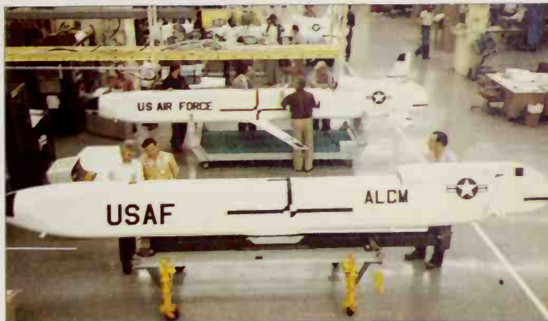
Inside the Seattle facility of Boeing Aerospace the long-range ALCM-B (AGM 86B) is seen in the foreground packaged for installation in or under a B-52. Beyond is the shorter ALCM-A, with everything for air-breathing cruising flight.
