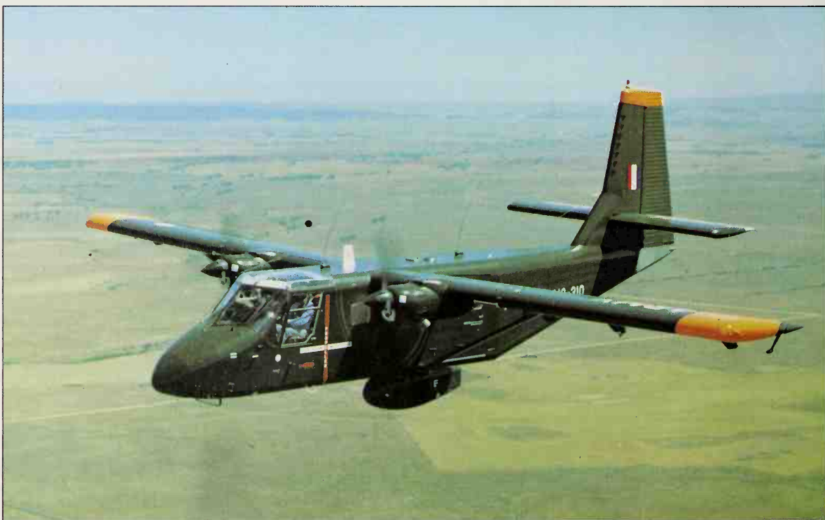
The GAF Mission Master is the military version of the N22B short-body model of the Australian twin-turboprop Nomad STOL transport. This 'MM' for the Australian Army has four wing pylons, transparent cockpit roof and comprehensive communications.
