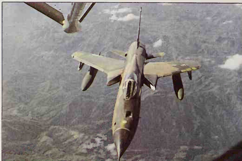
With nose receptacle open, this ANG F-105D is seen from a KC-135 tanker.
