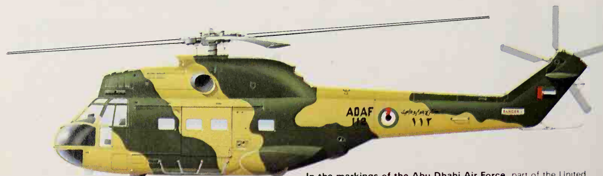
In the markings of the Abu Dhabi Air Force, part of the United Arab Emirates Air Force, this Aérospatiale SA.330 Puma is shown fitted with a sand filter in front of the engines for desert use
