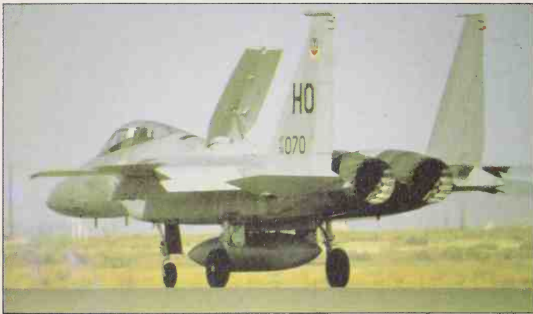
The F-15 Eagle has a clean exterior partly because all its EW/ECM systems were designed in from the start instead of hung on as afterthoughts. The chief system is Loral's immense ALR 56, which could hardly be fitted as a modification to any fighter.
