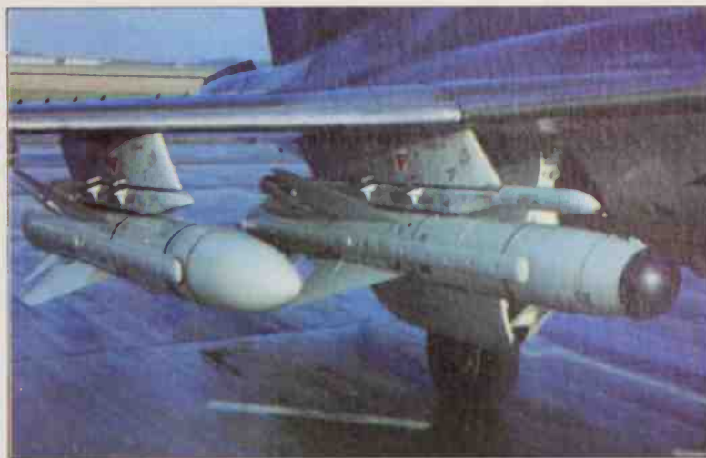
Under the right wing of an RAF Buccaneer S2B can be seen an AS 37 anti-radar Martel (left) and the British AJ-168 TV-guided version (right). Surprisingly, the French, who collaborated on both versions, never bought the more versatile 'British' version.
