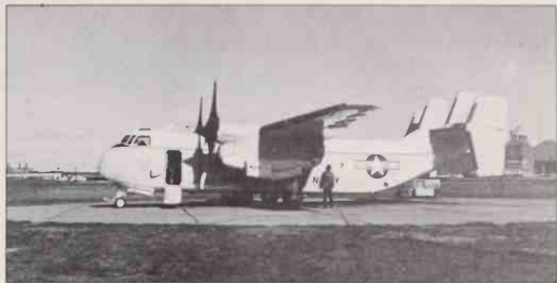
The Grumman C-2A Greyhound is a vital but lesser-known type in the US Navy's inventory. These COD (carrier on board delivery) transports are the lifeline between the Fleet and shore, and can make cat-takeoffs and arrested landings with 39 passengers.
