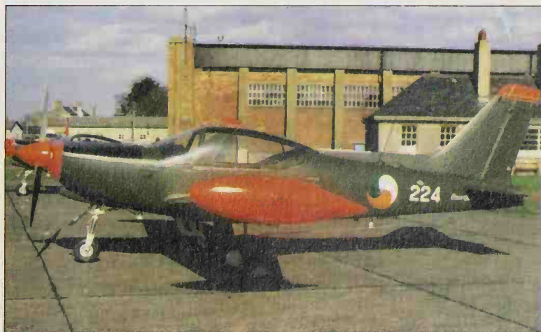
Most recent acquisition of the Irish Army Air Corps, ten SF.260WE Warriors provide economical multi-role and weapons capability well matched to the service's domestic needs. They are based mainly at the Casement HQ Airfield.
