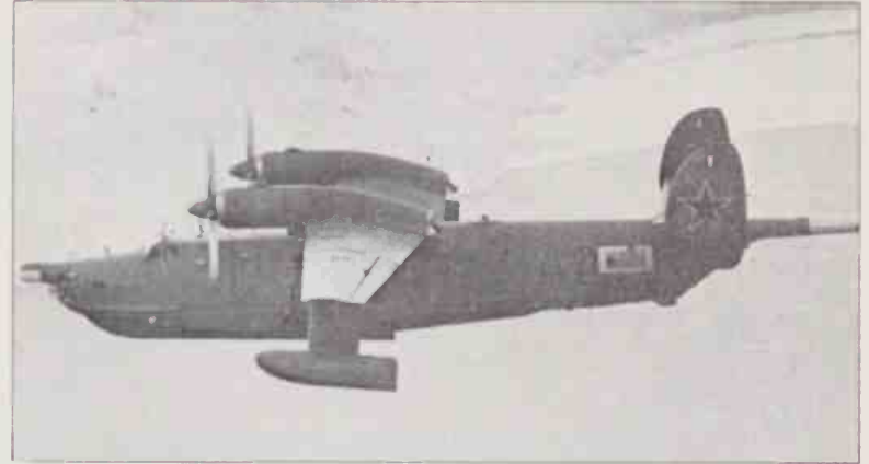
Called Tchaika (Seagull) by the Soviet AV-MF (naval air force), the Beriev M-12 (designated Be-12 by Beriev's design bureau) is a versatile turboprop amphibian.
