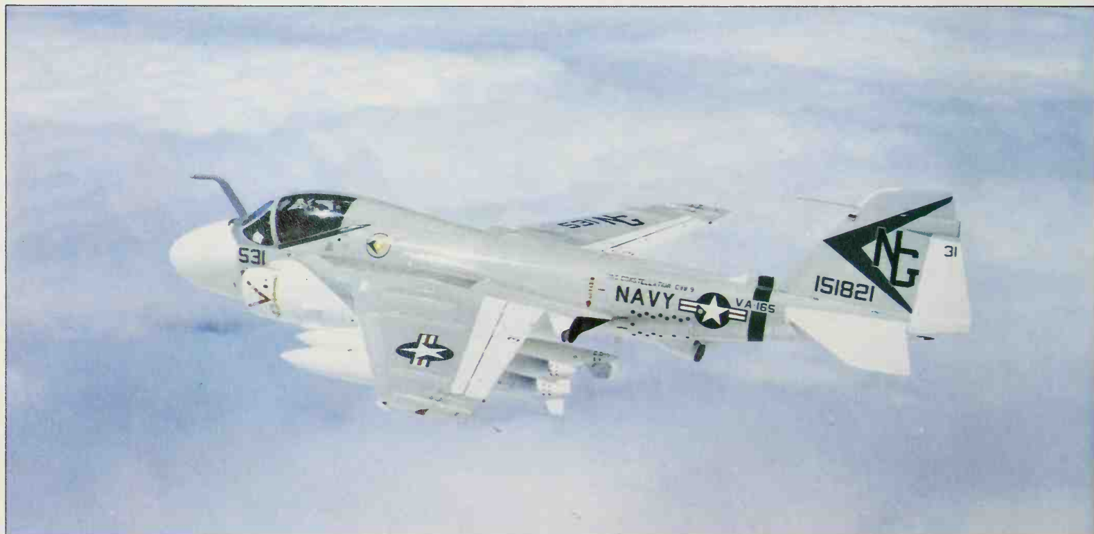
Grumman's KA-6D Intruder is the standard seagoing tanker of the 13 US Navy Carrier Air Wings. Distinguished chiefly by its hose-reel under the rear fuselage, it can transfer over 21,000 lb (9526 kg) of fuel; alternatively it can fly day attack or control missions.
