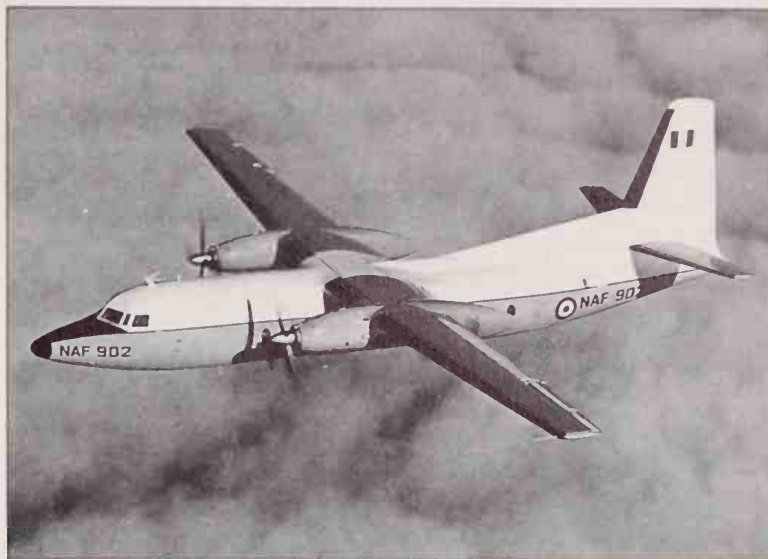
One of the users of the F27 Friendship military versions (at one time called Troopship) is the Federal Nigerian Air Force, which has two Mk 400 passenger/cargo transports equipped for parachute troops or airdrops from side doors.
