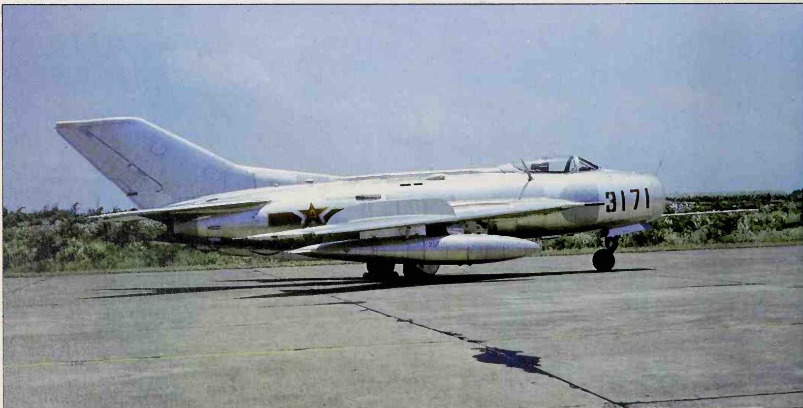
Though widely considered obsolete by the mid-1960s, the MiG-19 was a superb basic design with extremely low wing-loading and plenty of thrust and gun power. From it the Chinese derived this F-6, a tactical fighter subjected to progressive improvement, and the redesigned and much heavier Fantan, which the West calls F-6bis.
