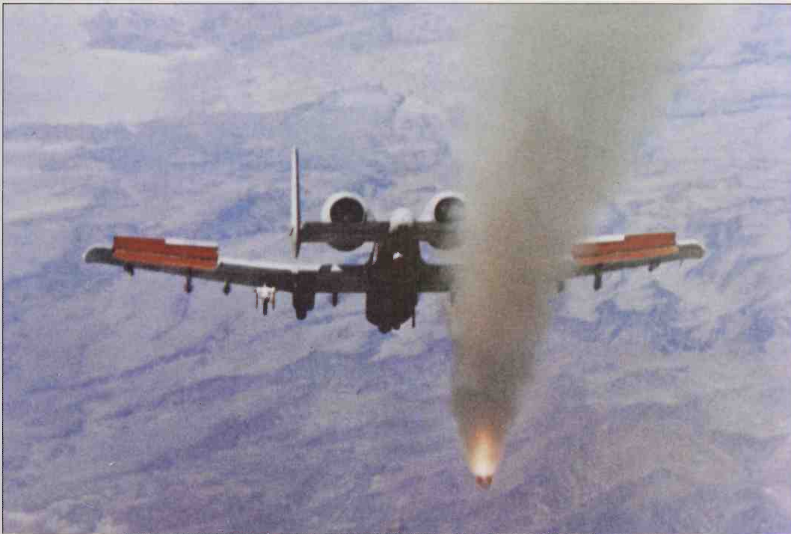
Taken during the type's flight development, this impressive photograph shows an AGM-65A Maverick precision air-to-ground missile being fired from a Fairchild Republic A-10A Thunderbolt II over a US range. Note the split ailerons opened above and below the wing for use as airbrakes.
