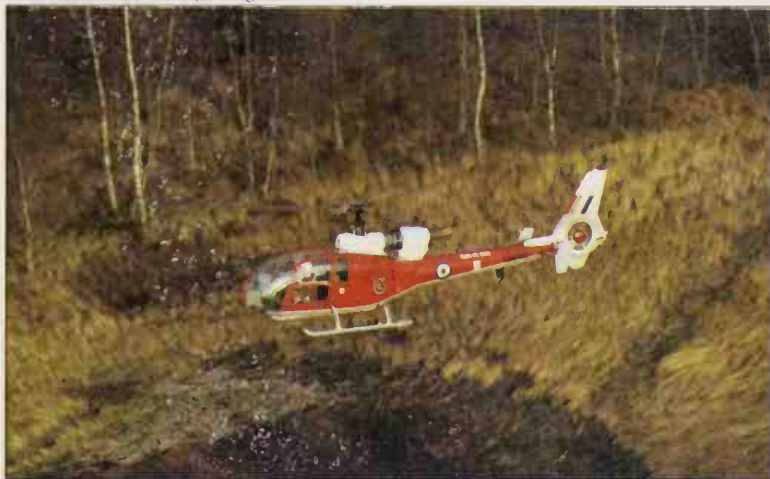
Aérospatiale SA.342 Gazelle with 'Fenestron' shrouded fan anti-torque tail rotor.
