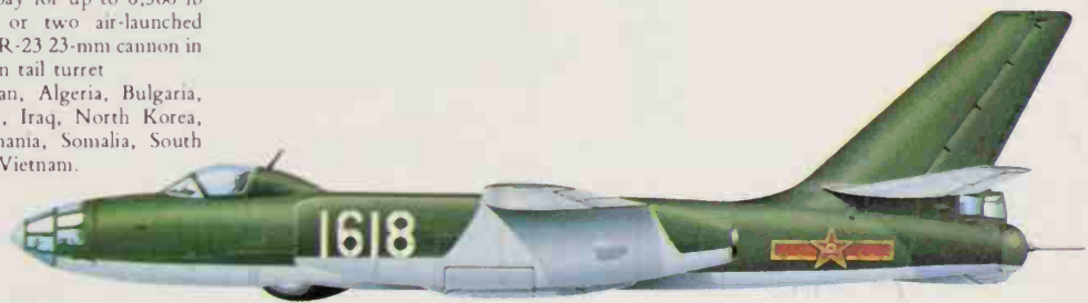
Chinese Air Force B-5 light bomber (Soviet Il-28 built under licence) of which more than 400 are in use
