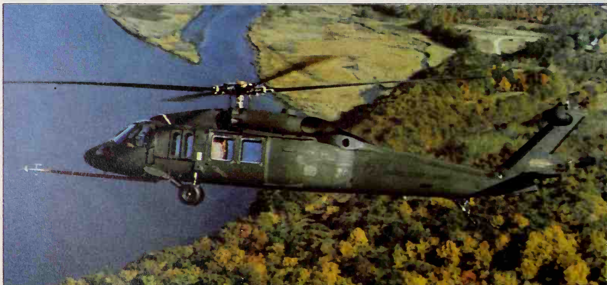
This prototype Black Hawk is distinguished by a long instrument boom carried ahead of the nose. The UH 60A development programme was the largest for any helicopter of the 1970s, the basic engineering task being multiplied by the need to meet severe numerical values for reliability and maintainability in harsh environments.
