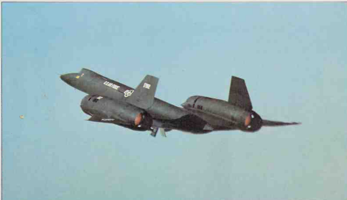
For 15 years the Lockheed SR-71 series of 'Blackbird' strategic reconnaissance aircraft have been the fastest military aircraft in the world. Supported by special-fuel KC-135Q tankers, they equip SAC's 9th Strategic Recon Wing at Beale AFB.
