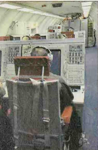
Operators seated at the MPCs (Multi-Purpose Consoles) of a Boeing E-3A Sentry AWACS (Airborne Warning and Control System), one of the most expensive production aircraft. The 552nd Wing at Tinker AFB has 20
