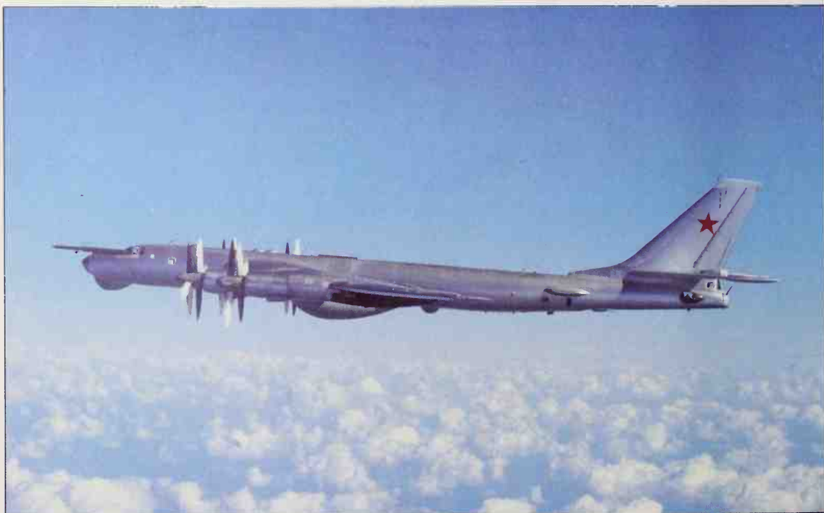
This Tupolev Tu-20 'Bear-D' was one of those intercepted almost every day near the British Isles by the RAF. Devoid of numbers or unit markings, it is packed with electronics for Elint, missile guidance and other duties. Endurance exceeds 24 hours, and some routine missions must reach close to this figure
