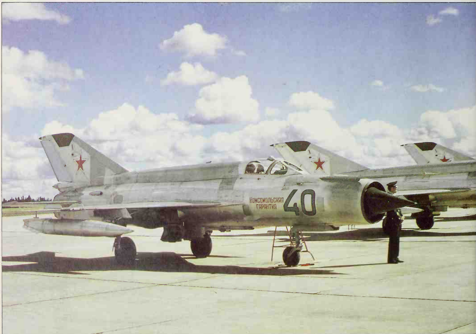
Late-model MiG-21s, apparently of the SMT sub-type called 'Fishbed-K' by NATO, seen on a rare visit outside the Soviet Union. This version has augmented avionics, with rear-warning radar, and fuel tankage restored to the large fuselage spine fairing.
