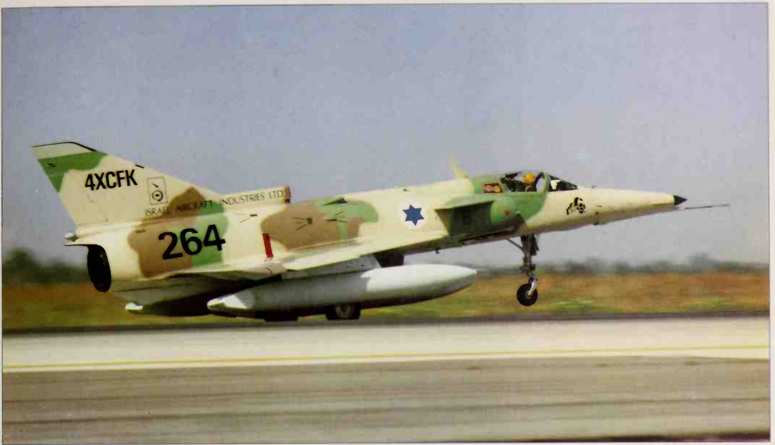
This Kfir-C2 lacks the M 2021 multimode radar and has instead the M-2001B ranging set which is limited to air/air or air/ground ranging of targets acquired visually. The large stores are finned drop tanks, though various ECM pods, bombs and air/air (Shafir) and air/ground missiles can be carried.
