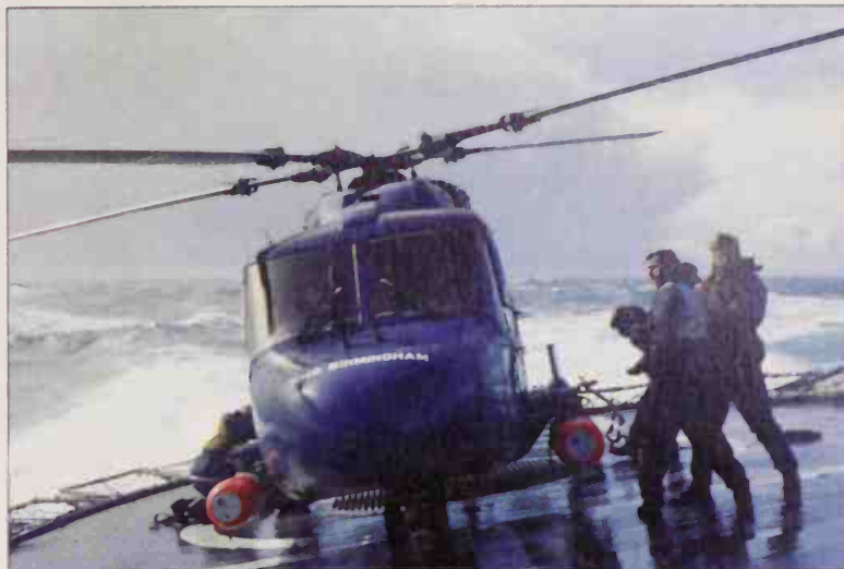
The Westland Lynx HAS.2 will soon be the most important helicopter in the navies of NATO, perfectly suited to all-weather multi-role duties on surface vessels. This Lynx, armed with Mk 46 torpedoes, is about to leave HMS Birmingham in a gale.
