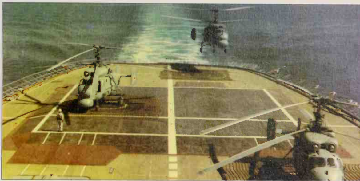
Still the standard shipboard ASW and missile-guidance helicopter of the Soviet naval air force, these Ka-25s are aboard the Moskva .
