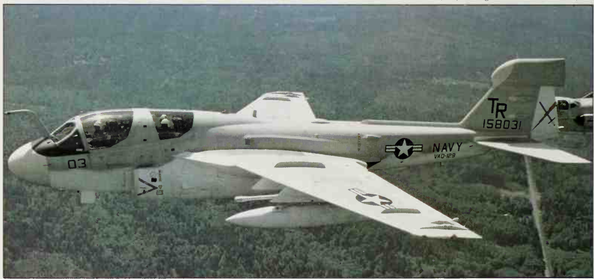
Grumman EA-6B Prowlers of US Navy carrier squadron VAQ-129 represent a high point in seagoing air technology. Their ALQ-99 ECM system costs more than the rest of the aircraft and is managed by two backseat operators. Five jammer pods can be added
