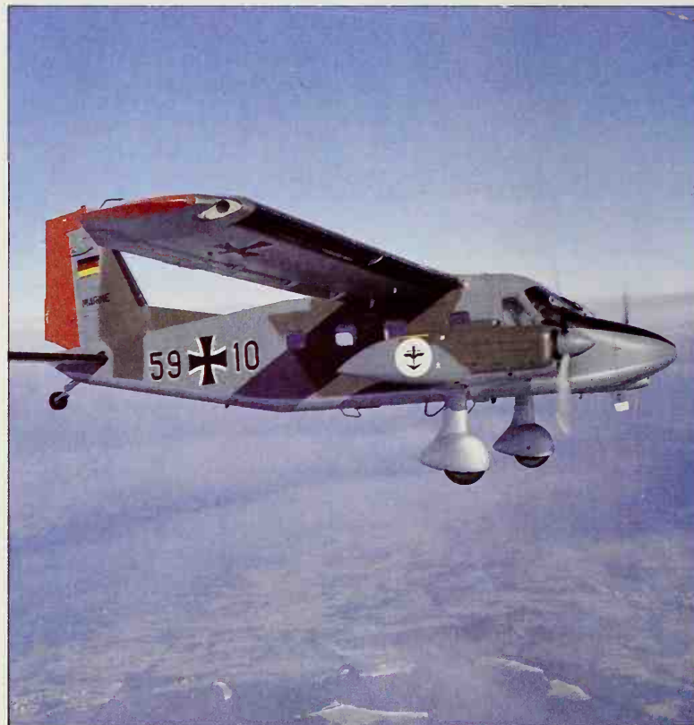
The Dornier Do 28D-2 Skyservant, here seen in service with the Federal German Marineflieger , is a STOL communications aircraft able to carry 13 passengers or a wide range of other loads. Dornier is trying to define advanced turboprop successors.
