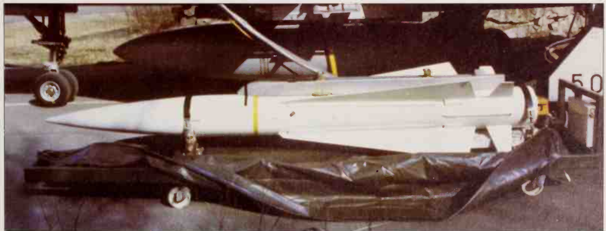
Saab's all-Swedish Rb05A is a simple command-guidance air/surface missile, here being mated to an AJ 37 Viggen. A more advanced TV-guided RB 05B was cancelled by the Swedish defence board, which bought the American Hughes AGM-65A Maverick instead.
