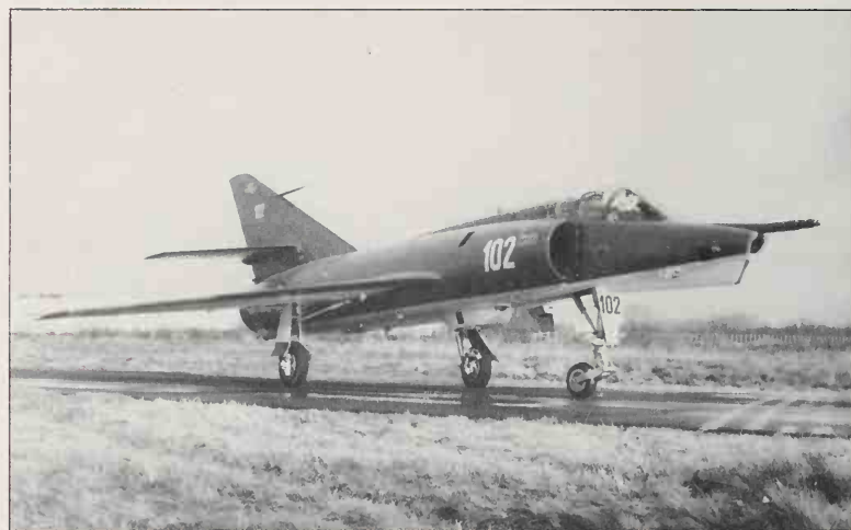
The Dassault Breguet Etendard IVP is an unarmed photo-reconnaissance aircraft which operates with the French Aéronavale from a shore base, Landivisiau, with Flottille 16F. Despite the Super Etendard the old IVP is likely to remain until at least 1985.
