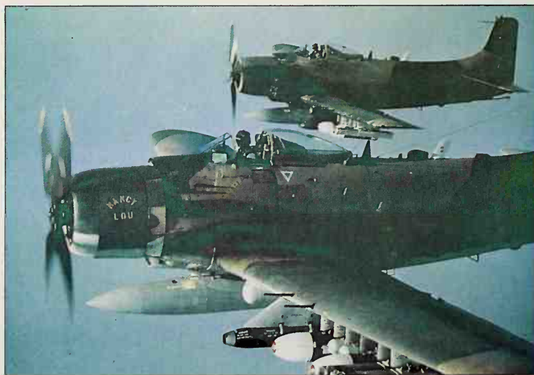
It has proved difficult to ascertain if any Skyraiders remain in genuine military service in 1980, though large numbers are still flying in several countries out of the 3,180 produced. These single-seat A-1H multi-role platforms of the USAF were escorting a 'Jolly Green' rescue helicopter in Vietnam, their pylons laden with weapons and equipment. One or two remain in US trials and research units.
