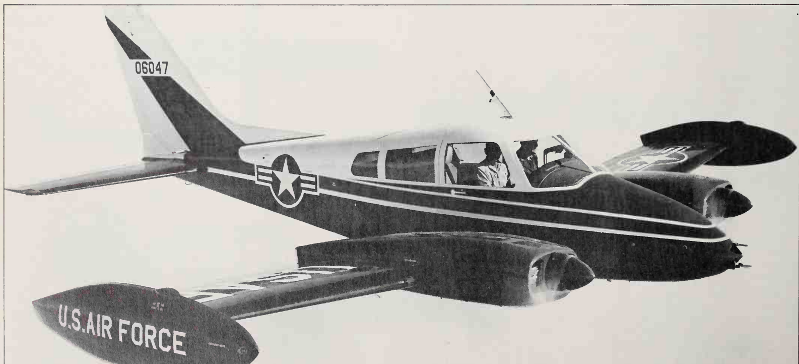
The Cessna U-3B is an administrative liaison and utility cargo transport for the US Air Force (36 delivered). Apart from having a swept fin, it is generally similar to the original U-3A (previously L-27A) model, of which 160 were bought in the late 1950s
