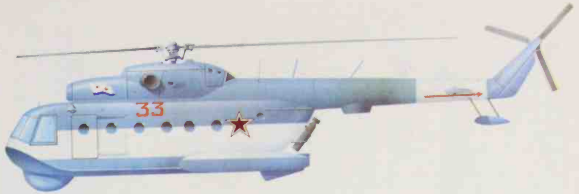
Becoming the standard shore-based Soviet Naval Aviation ASW helicopter, the Mil Mi-14 Haze-A has been developed from the Mi-8 Hip.
