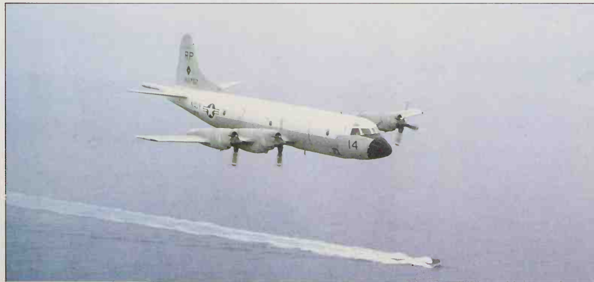
Lockheed P-3 Orion maritime patrol and anti-submarine warfare aircraft. Frequently updated and advanced avionics makes it possible to locate modern, deep-diving and quiet submarines against which the Orion can deploy a range of weapons
