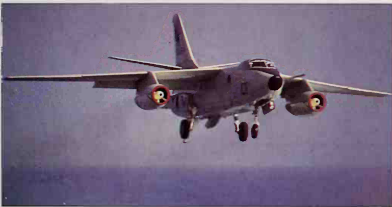
Designed to an exacting specification of 1948 for nuclear long range attack from carriers, the Skywarrior is still in use in unarmed KA-3 and EKA-3 form with Reserve units operating from a number of shore stations.
