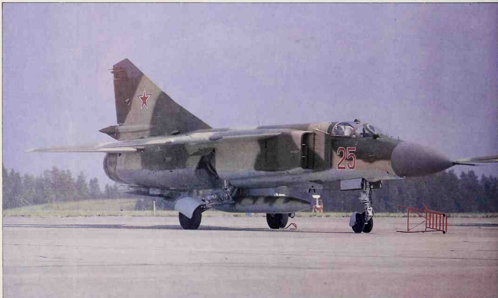
Still code-named 'Flogger-B' by NATO, this model of MiG-23S has a barely perceptible kink in the fin leading edge, extended-chord tabs on the tailerons, pylons for swing-wing drop tanks (usable at 16° sweep only) and, for foreign visits, no laser or AAMs.
