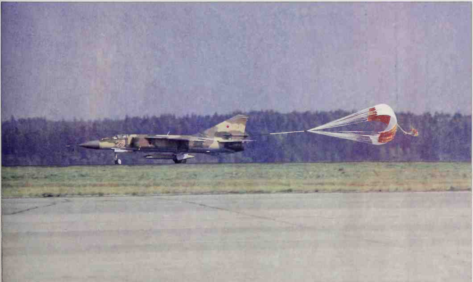
The MiG-23S of Soviet Frontal Aviation use a braking parachute of cruciform pattern—made from overlapping red and white rectangles. This one, landing at a Finnish airbase, is steering to the left with its mud-guarded nosewheels, with lower fin folded.
