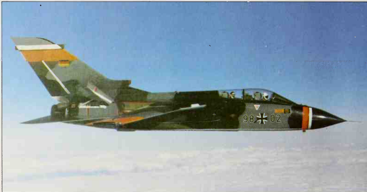
Now gradually becoming an important type in the West's armoury, the Tornado IDS is far more effective than any other aircraft of its size. This is No 13, a pre-production example, forming with speedbrakes open to kill speed.
