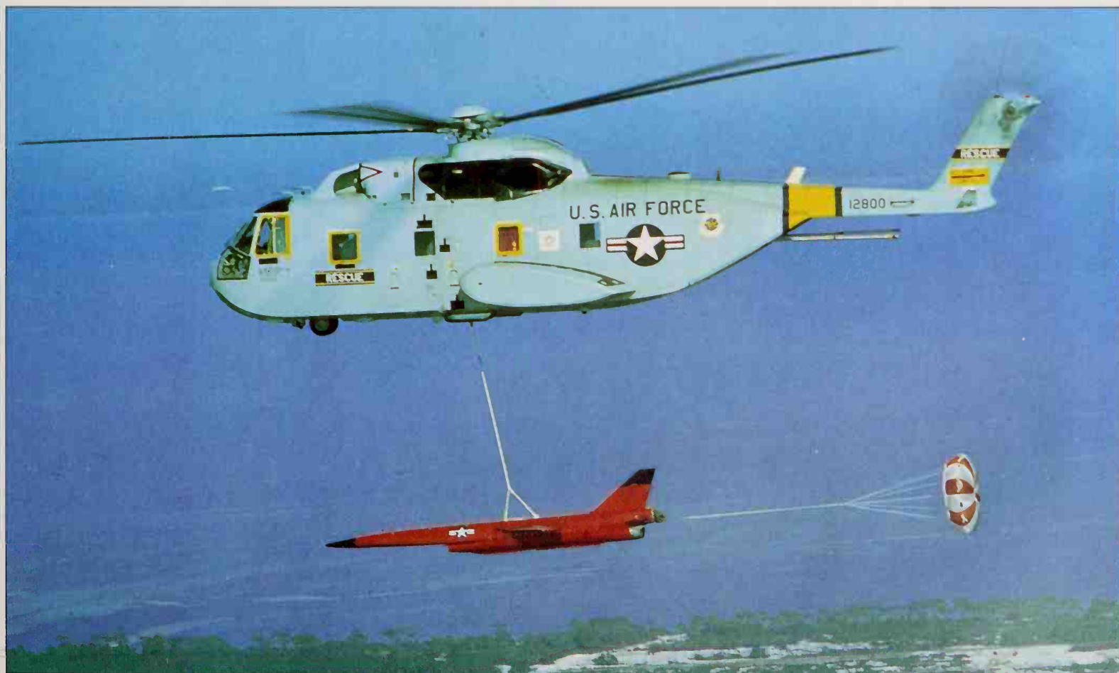
A Sikorsky HH-3E, of the nosewheel/rear-door S-61R species of the USAF Aerospace Rescue & Recovery Service, retrieves a BQM-34C Firebee II supersonic RPV target during the November 1976 William Tell annual Fighter Weapons meet at Tyndall AFB.
