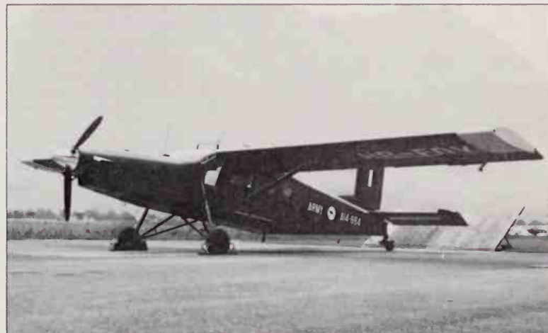
The Pilatus PC-6/B Turbo-Porters used by the Australian Army Aviation Corps are powered by the Pratt & Whitney Canada PT6 turboprop (other models have Turbomeca or Garrett engines). The AAAC has 18, serving with units at Oakey and Holsworthy.
