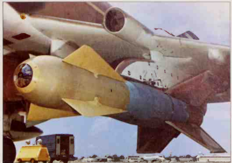
Developed under the USAF Pave Strike defence-suppression programme, this CWW (Cruciform-Wing Weapon) is designated GBU-15 (V) and adds precision electro-optical guidance to a large M118 bomb. Carrier in this case is an F-4E Phantom of TAC
