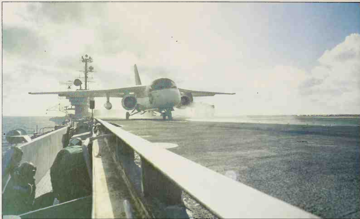
Lockheed S-3A Viking anti-submarine aircraft attached to the USS Saratoga. The four man crew of each Viking has available the most advanced sonobuoys and MAD equipment to seek out the quieter, deeper-diving submarines which are currently in service with major powers
