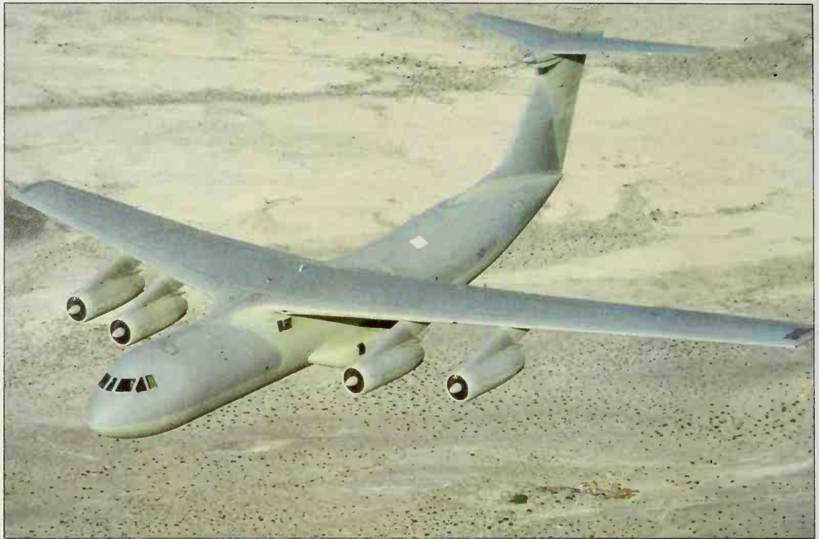
All Lockheed C-141A StarLifter strategic airlifters were delivered in natural metal finish, but in December 1977 this example tested a low-visibility paint scheme. It may become standard, as will the long body and other improvements of the C-141B.
