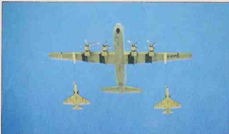
One of the many home-produced success stories of the Israeli Heyl Ha'Avir is the rebuild of several Boeing 377 Stratocruisers as multi-role military freighter/tankers, since supplemented by ex-USAf KC-97s
