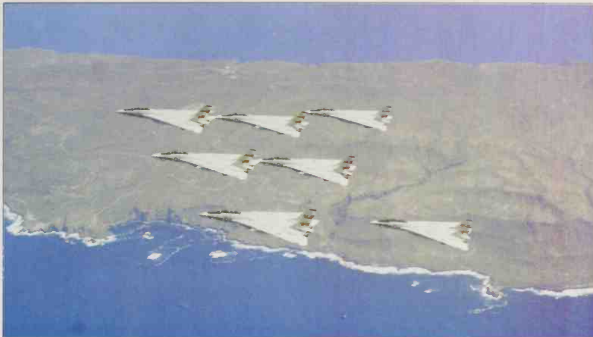
Seven Grumman F-14A Tomcats, all in tight formation with wings at 68°, present an impressive and unusual sight because this sweep angle is seldom chosen in subsonic regimes. This part squadron comes from CVA 65 Enterprise , the first nuclear carrier.
