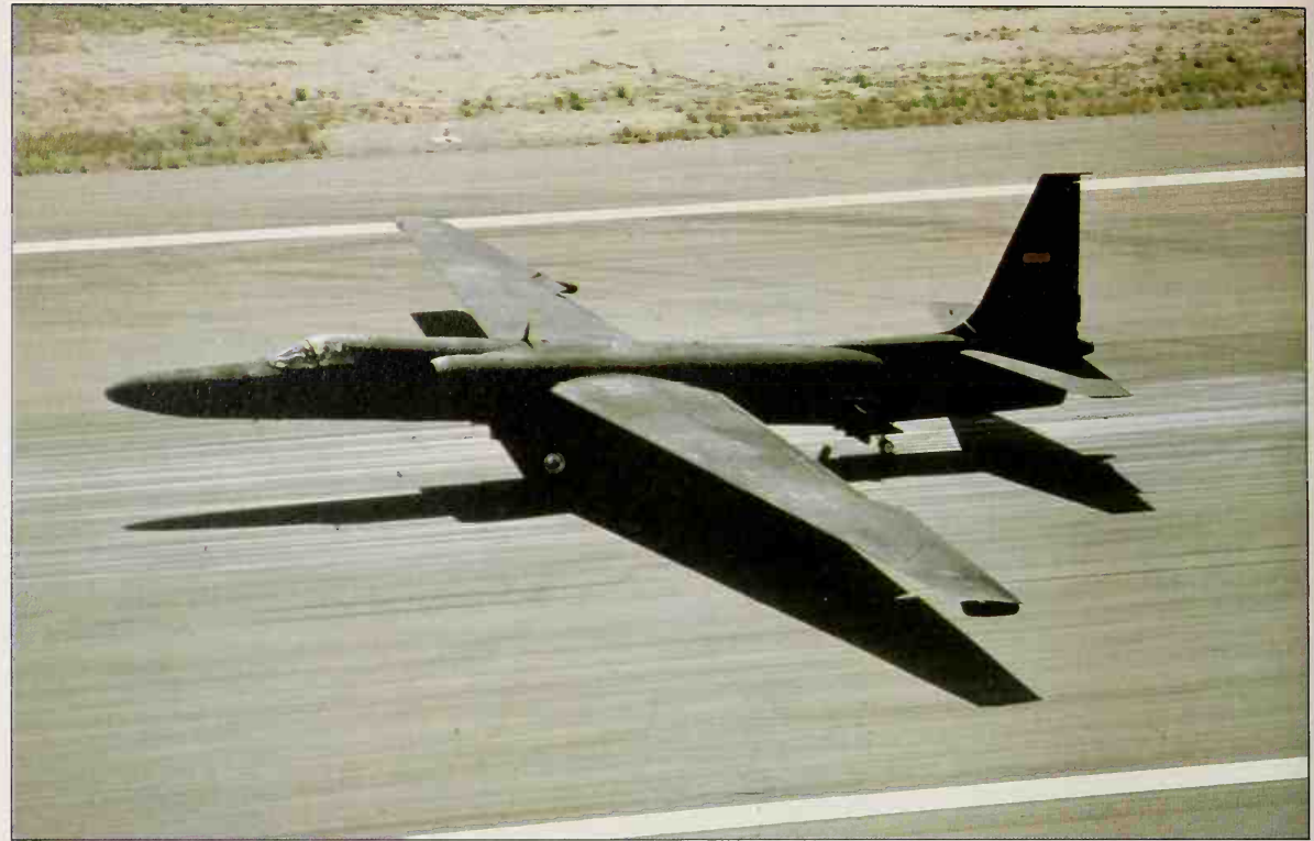
This dark stranger is a Lockheed U-2R, much larger than other versions of the clandestine U-2 mystery ship and in this case operating in black out of Davis-Monthan AFB with no marking save tail-number 10333 in red. This airframe is the basis of the TR-1.
