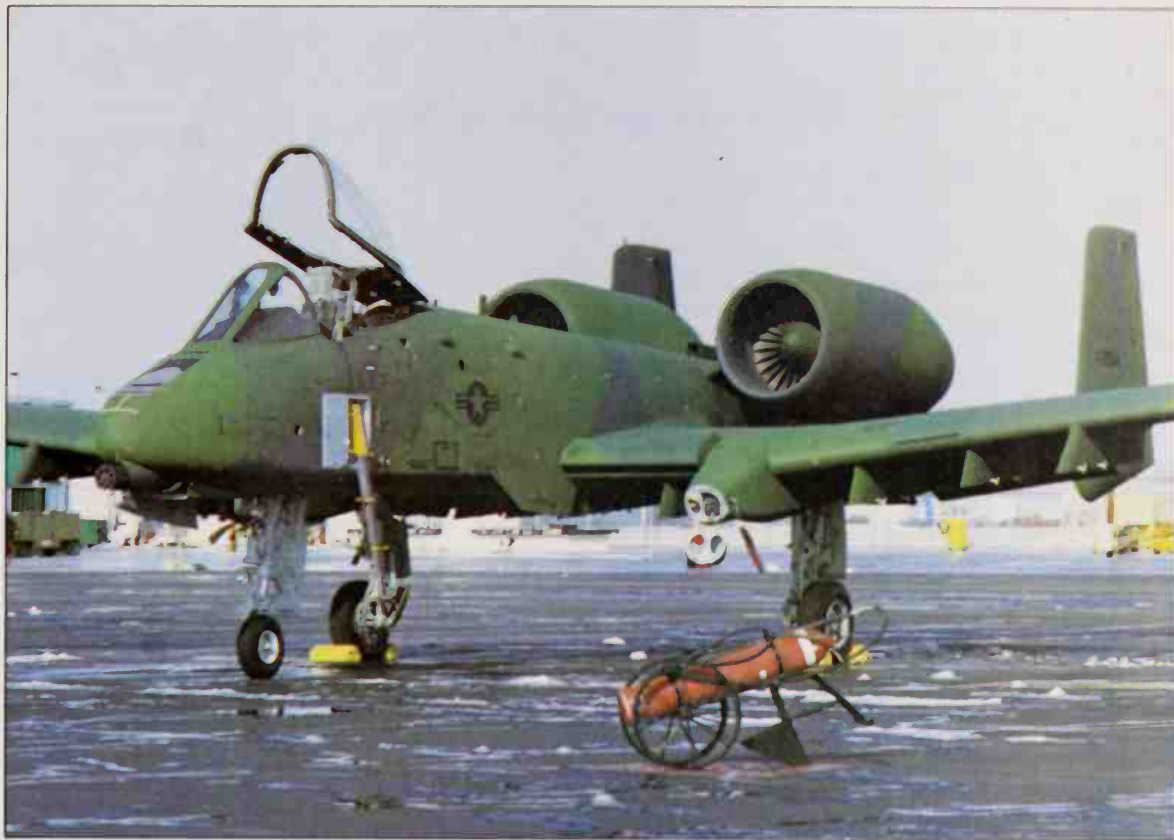
This so-called lizard camouflage is now standard in Tactical Air Command A-10 units, in place of the overall grey previously used. This aircraft, which does not have unit insignia, has the pilot ladder extended.
