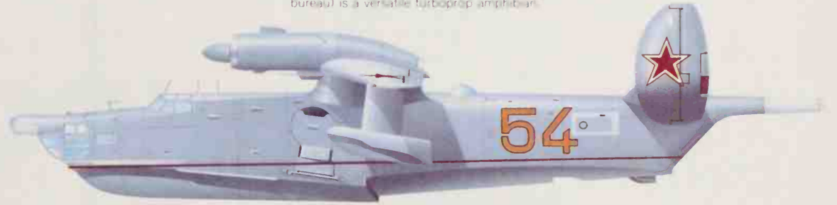
The Soviet Naval Air Force or AV-MF still operates a number of Beriev Be-12 Mail medium-range maritime patrol amphibians.
