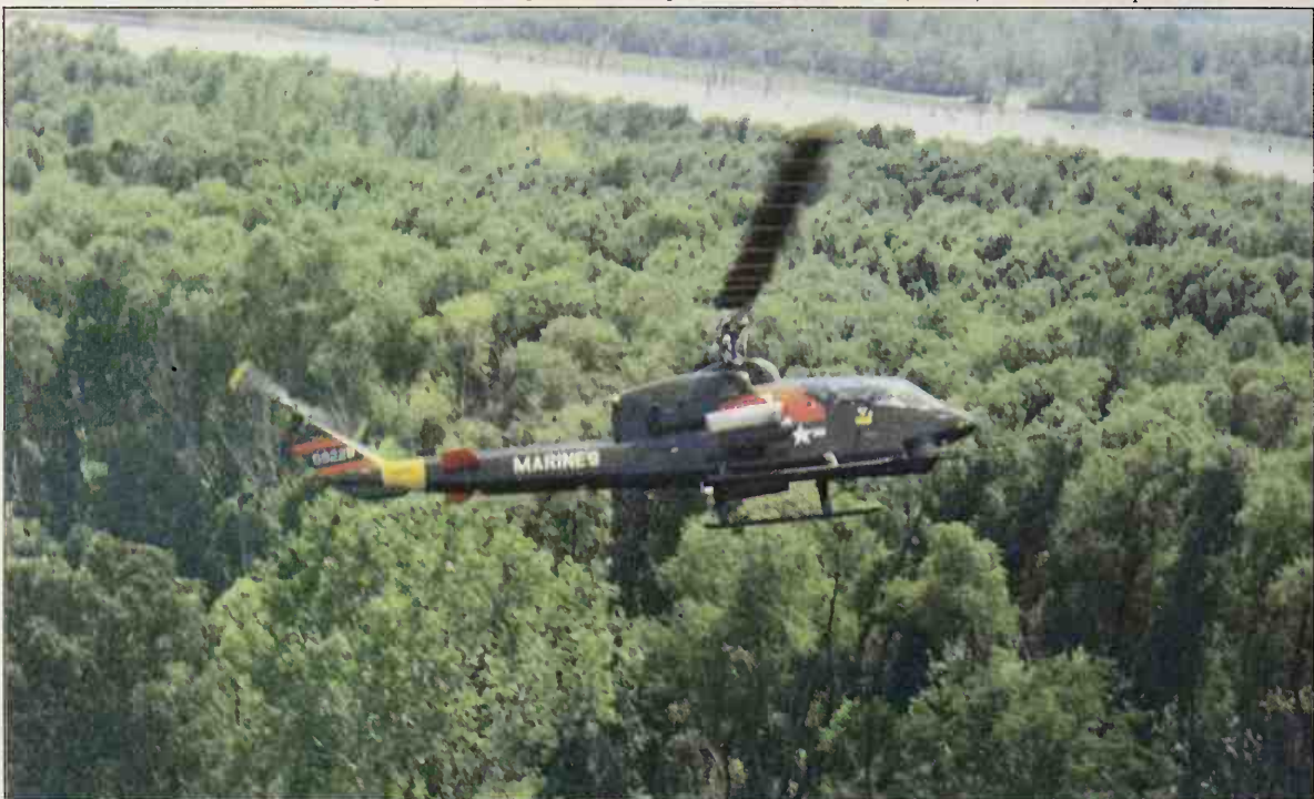
Bell AH-1T SeaCobra , known also as the Model 209 improved SeaCobra, which has been developed from the twin-engine AH-1J SeaCobra. Ordered for the US Marine Corps, these helicopters have an uprated powerplant, a new dynamic system and advanced technology features.
