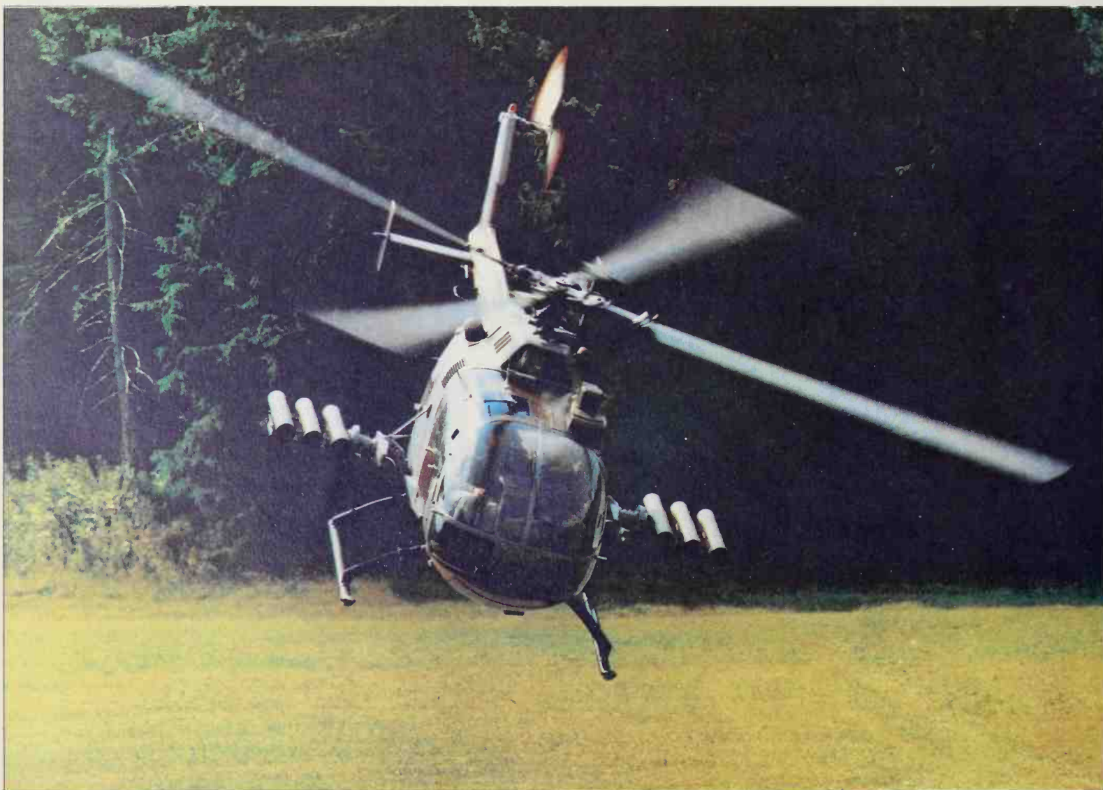
Designated PAH-1 (for anti-armour helicopter Type 1) by the Federal German Heer (army), the MBB BO105P can carry six of the Euromissile Hot anti-tank weapons and the complex associated sight and tracking system. A total of 212 are being delivered at six per month. Meanwhile bids for a successor PAH-2 were being studied in late 1979.
