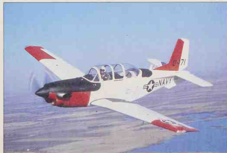
Beech T-34C, two-seat turboprop-powered primary trainer, for service with the US Navy. Developed in 1948 from the civil Bonanza, it was used extensively as a piston engine trainer until conversion to turboprop power in 1973 brought new orders
