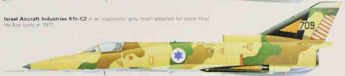
IAI Kfir without foreplanes and sporting tactical camouflage fitted with the simple Elta ranging radar. The rudder striping was previously carried by an IAF/DF Mirage IIICJ unit.
