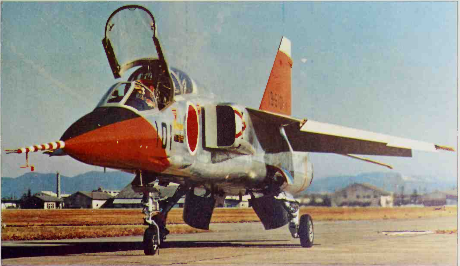
This neat machine, closely modelled upon the similarly powered Jaguar, was the original prototype Mitsubishi XT-2 trainer, flown in July 1971. From this have been developed not only the production T-2, standard supersonic trainer of the JASDF, but also the single-seat F-1 multi-role fighter
