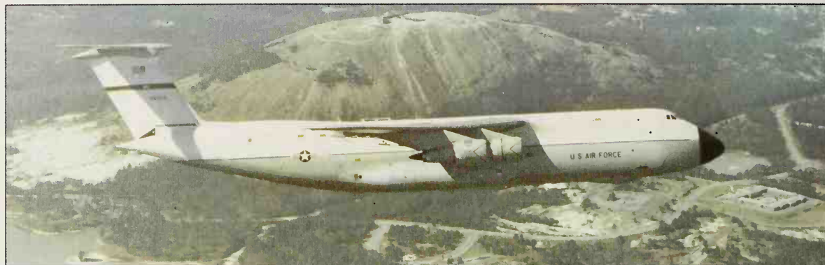
By far the largest military transport in service with the West (unless an airlift version of the 747F were to be developed), the C-5A is a crucial item in NATO planning despite prolonged structural problems that have come to a head in the decision to build new wings for all aircraft in service. The basic USAF Military Airlift Command force numbers 76, in four squadrons.
