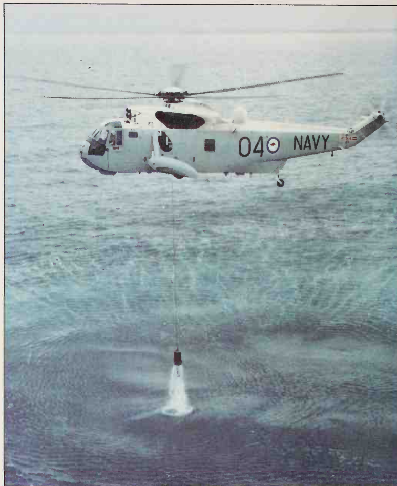
Dunking a sonobuoy, the Westland Sea King 50 is the standard ASW helicopter of the RAN's Fleet Air Arm Air Group, serving with HS 817 squadron. The Mk 50 was first of the updated series of Westland Sea Kings.
