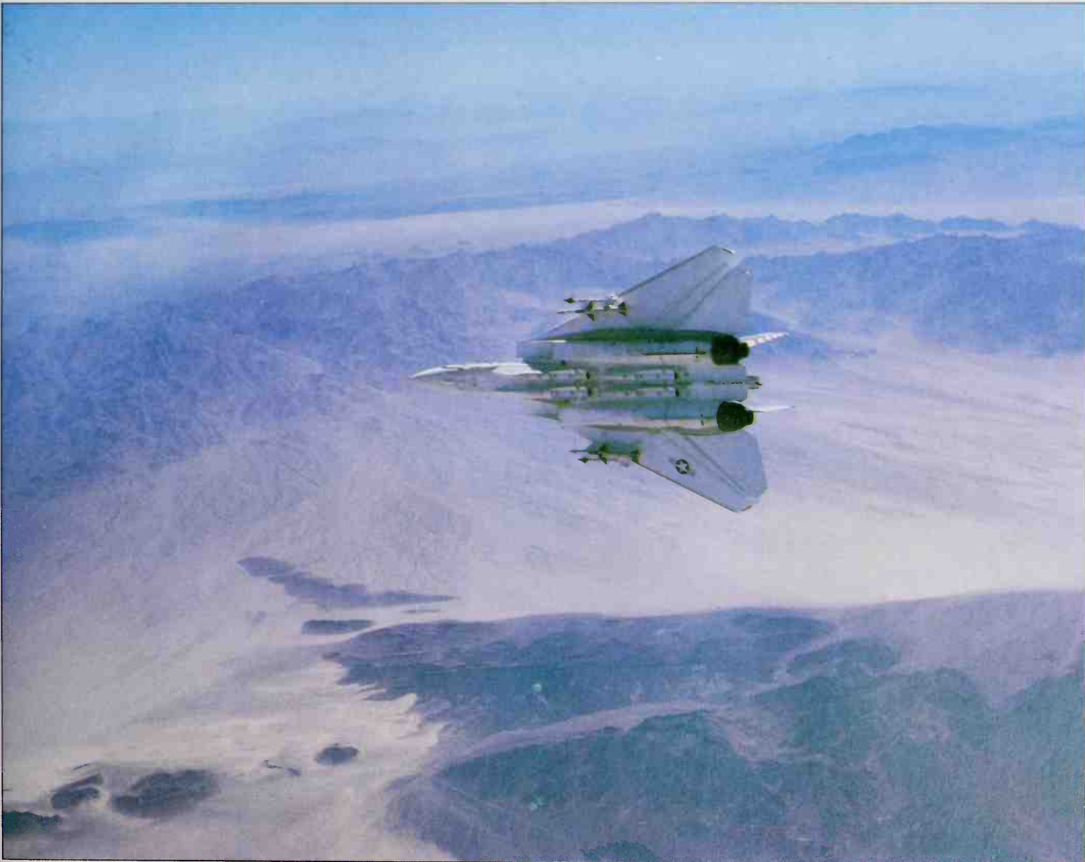
This Grumman F-14A Tomcat is probably operating out of NAS Miramar in southern California, but appears to have tail insignia of USS Constellation . It is fully armed with four long-range Phoenix, two medium-range Sparrows and two close-range AIM-9s.
