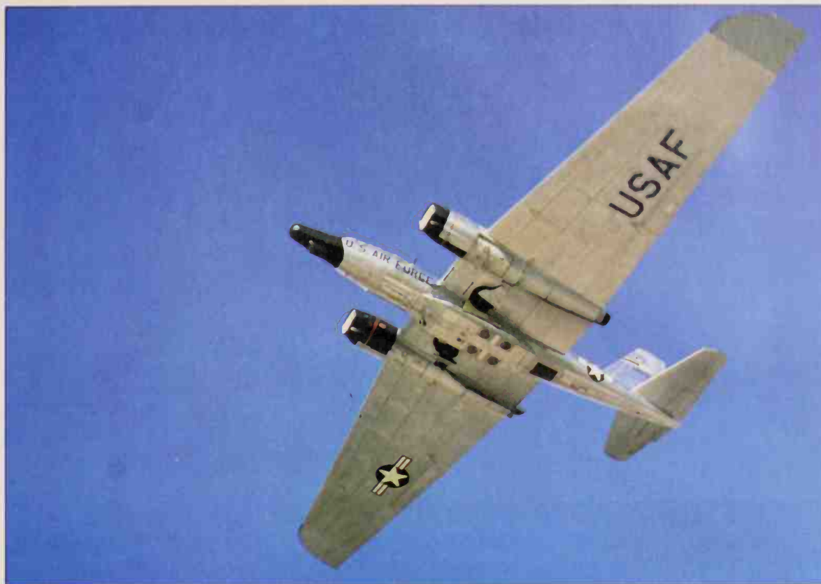
This grotesque WB-57F was developed from the British Canberra by Martin and General Dynamics for extreme altitude reconnaissance. This one was assigned by the USAF to NASA for Project Airstream, sampling nuclear radiation, Howard AFB, Canal Zone, 1977
