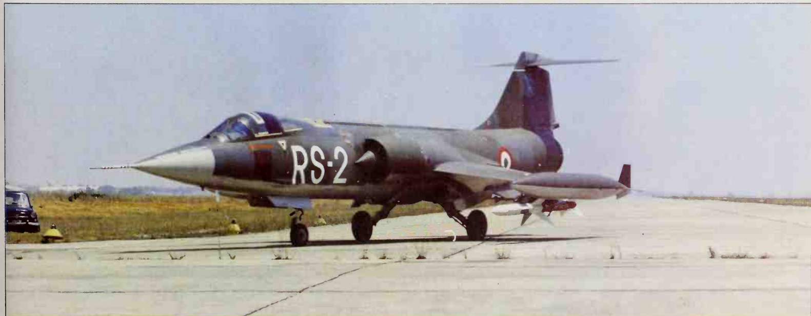
This Aeritalia F-104S Starfighter was one of the test fleet selected to complete development and service indoctrination trials with the Aspide, a medium-range AAM derived from the American Sparrow but claimed by the Italians to have numerous improved features. By 1980 the Aspide 1A should be entering combat service replacing the AIM-7E Sparrow
