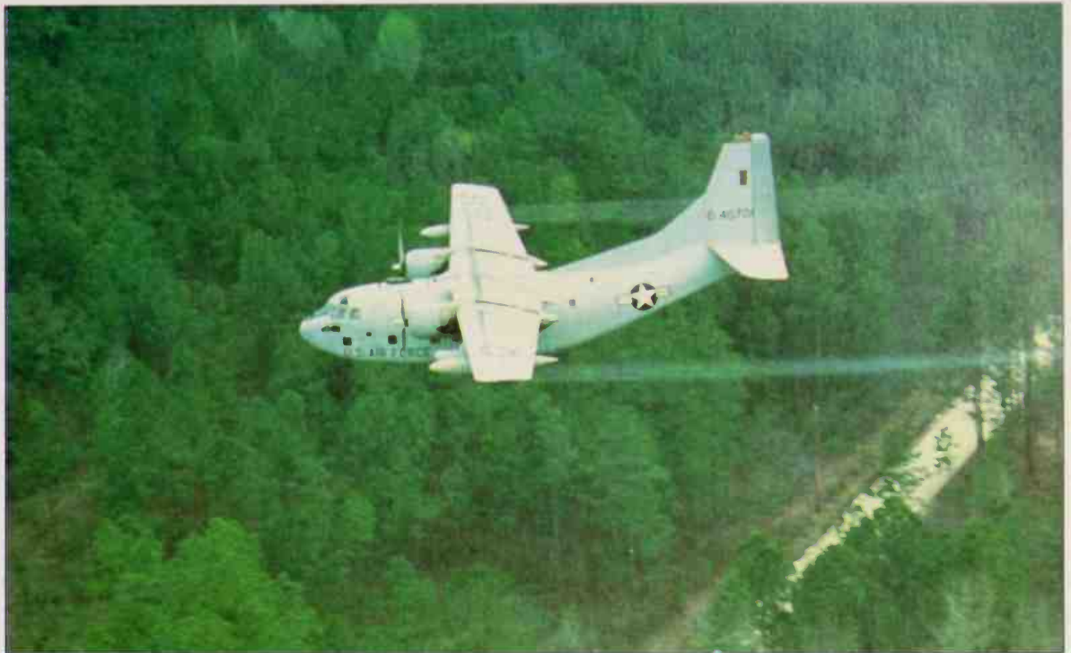
This Fairchild C-123K Provider was photographed in March 1976 during spray training at Fort Stuart, Georgia. The Provider was the type used to defoliate vegetation in Vietnam to try to deny cover to the Viet Cong. Training was carried out with water.
