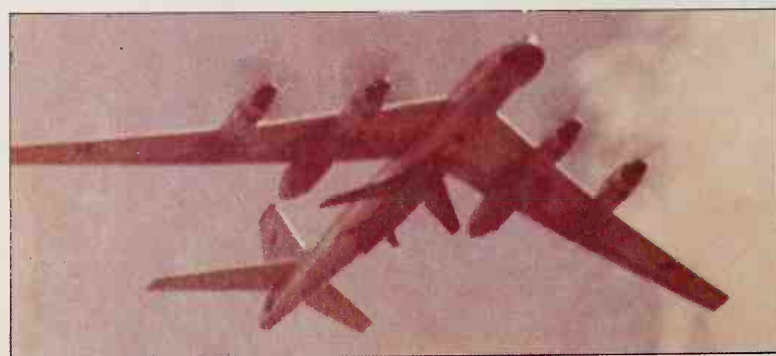
Called AS-3 'Kangaroo' by NATO, this air/surface missile carried by the so-called 'Bear-B' and 'C' versions of the Tu-20 is the largest air-launched weapon ever developed in numbers.
