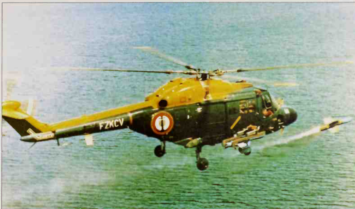
Due for replacement by the wire-guided AS.15 in the early 1980s, the obsolescent AS.12 is still in service with French helicopters including the Lynx of the Aéronavale as seen here. TCA guidance is not available on AS.12.
