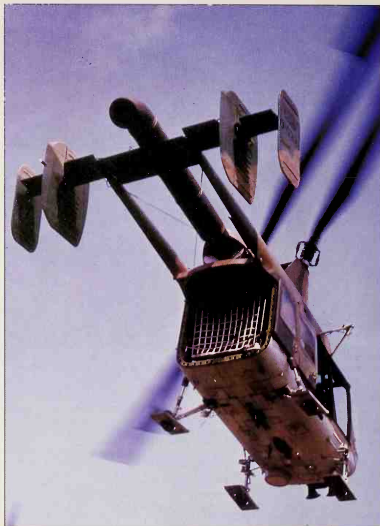
Last of the 'egg-beaters' with Kaman-style intermeshing rotors, the HH-43 Huskie is still used by several air forces. This example was pictured on jungle rescue duties in South Vietnam in 1967 with Detachment 12, 39th USAF Aerospace Rescue & Recovery Sq.
